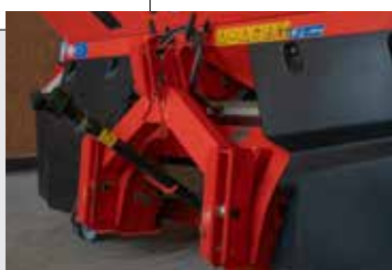
Retrofittable weighing frame for remaining quantity display
