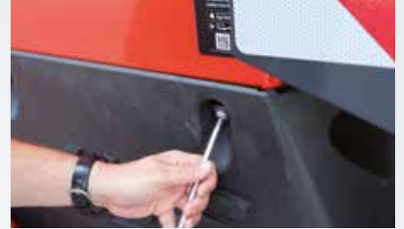
Dirt deflector with quick release fastener
