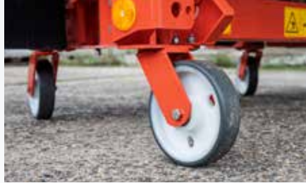
Parking rollers with quick release coupling system
