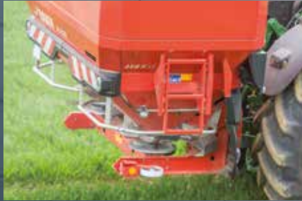
AXIS H –Right and left full border spreading via rotation speed and drop point adjustment
