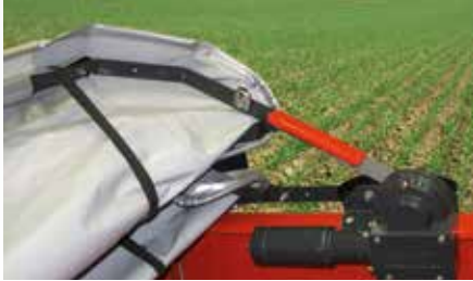
Electrically remote-controlled hopper cover
