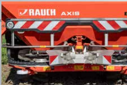
Limited border spreading unit GSE pro
