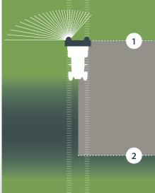
The weighing spreader requires a very long time to react. Both slides are adjusted simultaneously.
