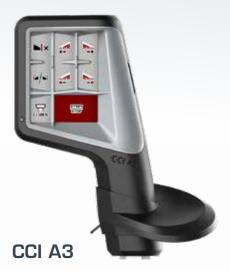
After plugging in the AUX N interface, the corresponding symbols for operating the unit are shown on the small touch screen. The driver can thus always see which functions he/she has stored here.
