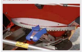
The easily readable, quantity-proportional DfC scale, unique to RAUCH, allows reliable quantity corrections after a calibration run.
