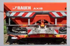
Limited border spreading unit GSE 30/60
