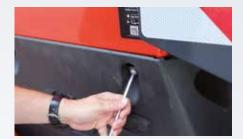
Dirt deflector with quick release fastener
