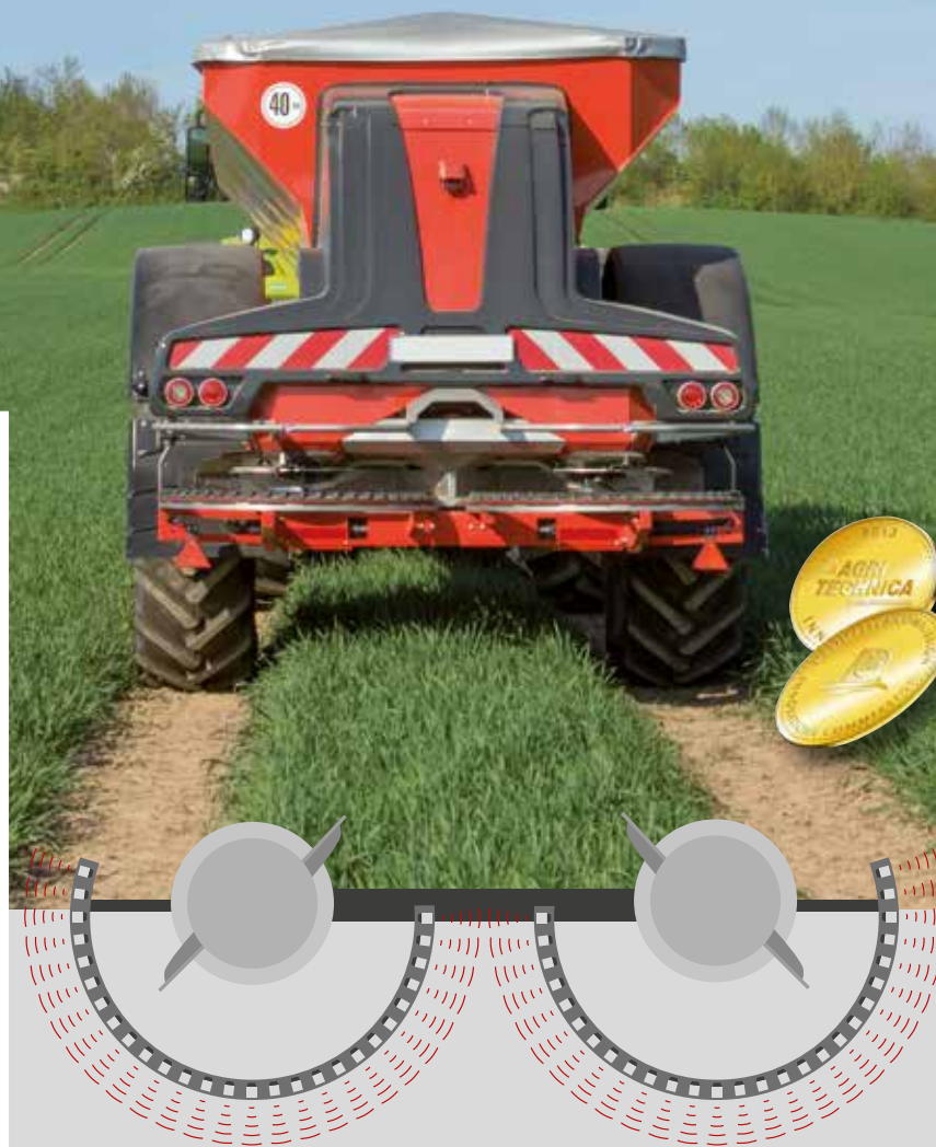
Precise spreading pattern analysis via 54 radar sensors
