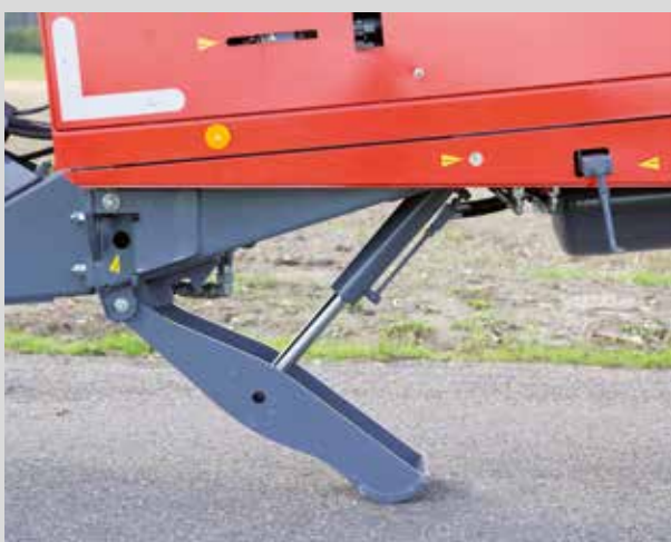
The hydraulic support stand ensures quick and reliable stabilisation
