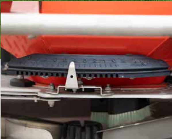
High ease of use due to electric drop point adjustment for a variable section adjustment (optional)
