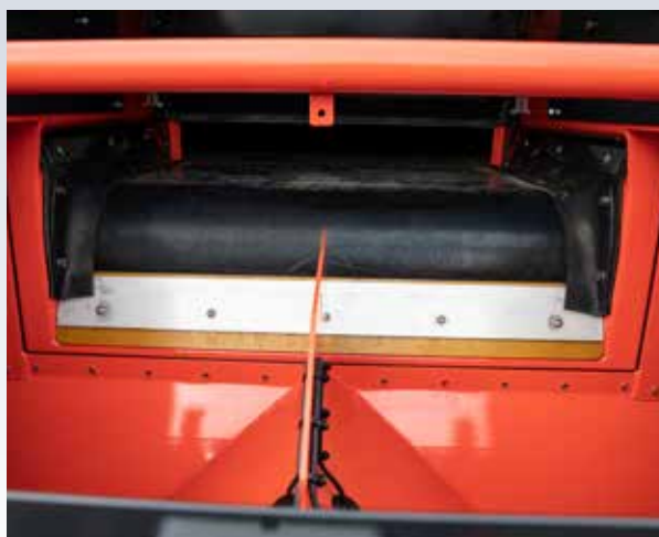
Conveyor belt with belt scraper
