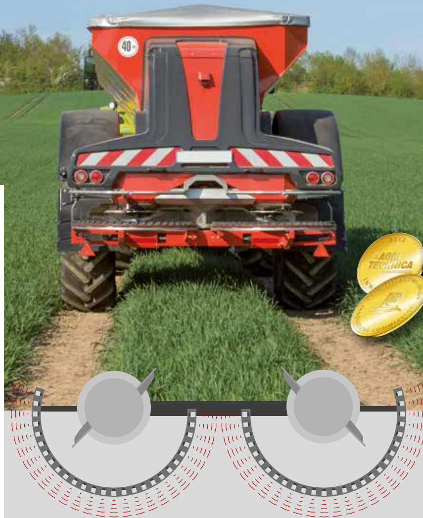
Precise spreading pattern analysis via 54 radar sensors
