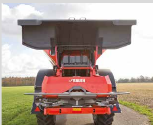
Maintenance flap with gas pressure spring
