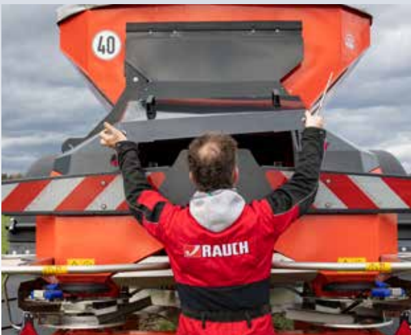
The cover of the spreader unit can be removed for easy cleaning of the machine.
