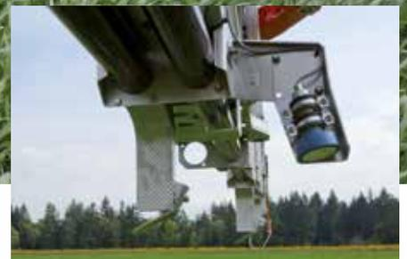
Distance Control: Ultraschallsensor
