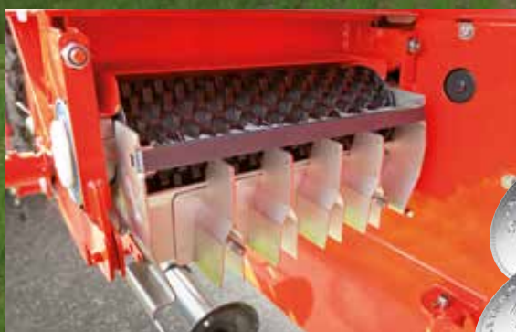
One metering unit per section
