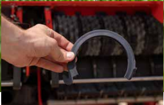
Nitrogen metering roller with fine metering kit
