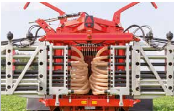
Pendulum frame suspension
