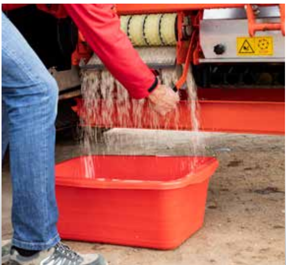
Residual quantity discharge
