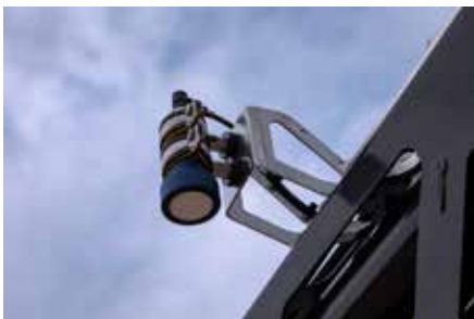
Distance control: Ultrasonic sensor
