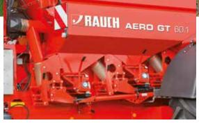
Three separately adjustable metering units on each side
