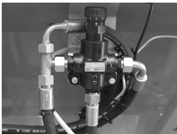
Figure 6.10: Flow control valve
