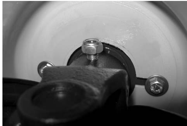
Figure 6.6: Tighten the hexagonal screw.
