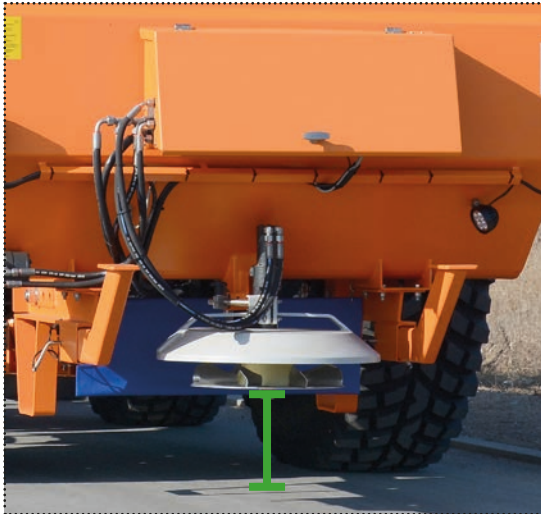
Working height: Spreading disk 35 to 45 cm above ground
