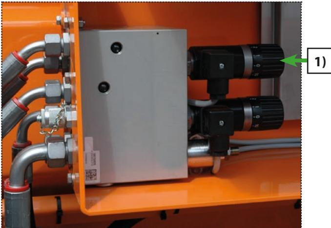
Abb.: Hydraulikblock SRCA 2-fach
