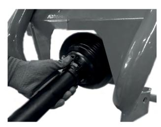
Fig. 14: Mounting the universal drive shaft cover
