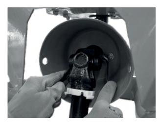
Fig. 13: Connecting the universal drive shaft
