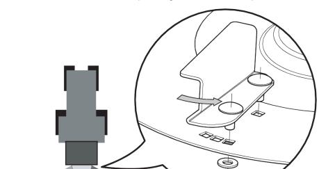
Dismount the screws of the spreading vanes with the respective nuts and washers.
