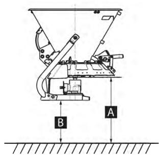
Fig. 16: Setting the mounting height
