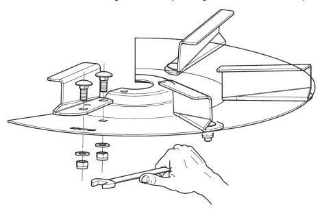
Fig. 29: Loosening the screws of the spreading vane
