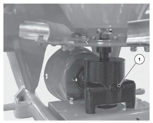
Fig. 31: Checking screw for transmission oil level
