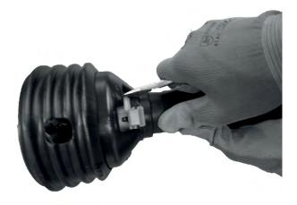
Fig. 11: Opening the universal drive shaft cover
