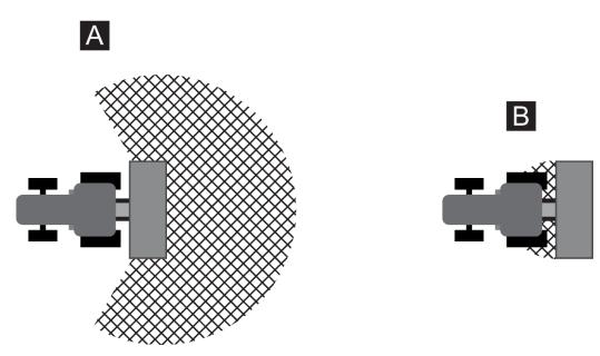
Fig. 1: Hazard zone when devices are attached
