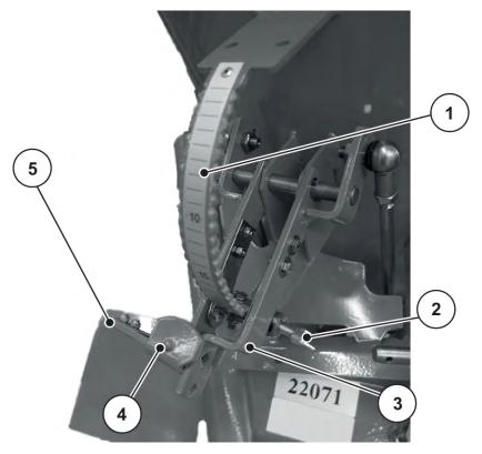
Fig. 23: Scale for adjusting the application rate
