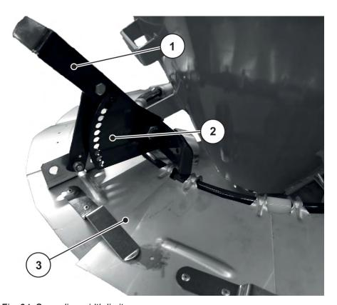
Fig. 24: Spreading width limiter
