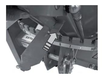
► Turn the adjusting element in the desired direction.
