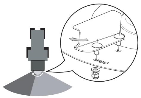
Fig. 23: Spreading density on the right in direction of travel
