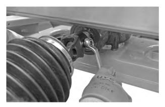
Fig. 15: Connecting the universal drive shaft
