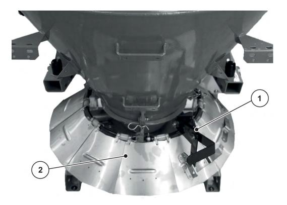
Fig. 26: Spreading width limiter setting
