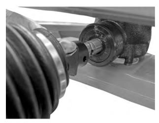
Fig. 14: Pushing the universal drive shaft onto the transmission spigot
