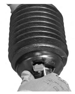
Fig. 13: Opening the universal drive shaft guard
