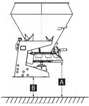
Fig. 19: Setting the mounting height
