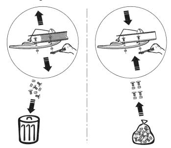
Fig. 36: Using new self-locking nuts
