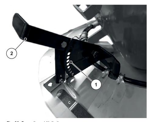
Fig. 30: Spreading width limiter
