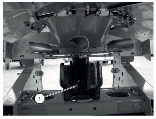
Fig. 39: Transmission oil level checking screw
