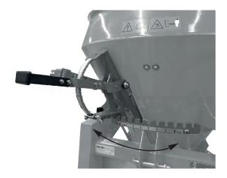
► Insert the locking mechanism in the desired position.
