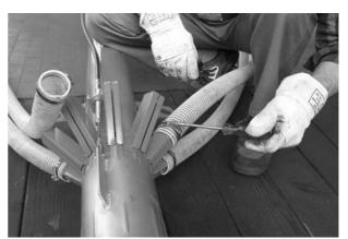
**3.** Fasten the hose clamps tightly onto the profiles.
