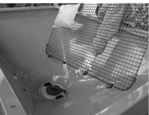
Figure 5.3: Remove the protective grid
