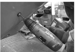
1. Remove the bracket clamp screws (4x).
