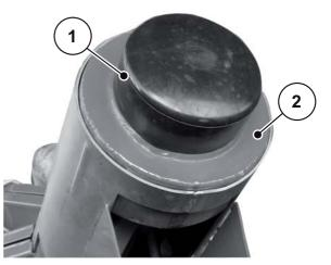
1. Remove the upper pipe plug cap [1] from the screw tube [2].
