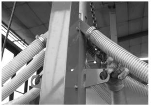
Figure 9.1: Attach the lifting gear to the screw tube
