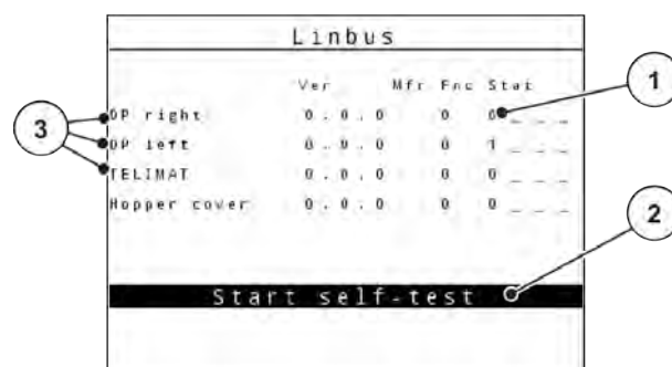
Fig. 44: Test/diagnosis; example: LIN bus
