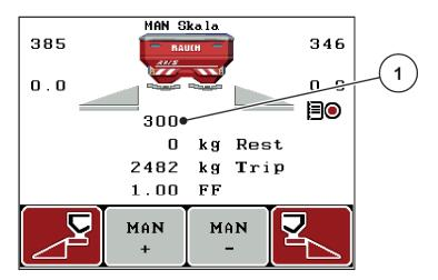
Fig. 35: Operating screen MAN scale
