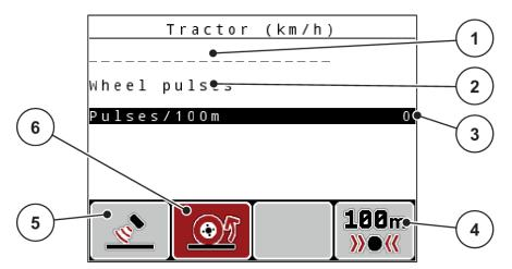
Fig. 33: Tractor (km/h) calibration menu
