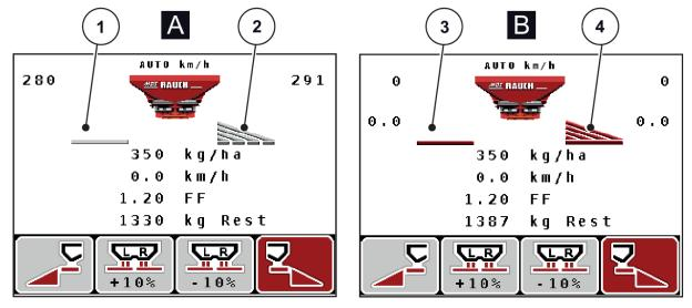
Fig. 7: Display of the MDS metering slide status
