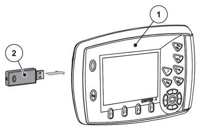
Fig. 50: Inserting a USB stick
