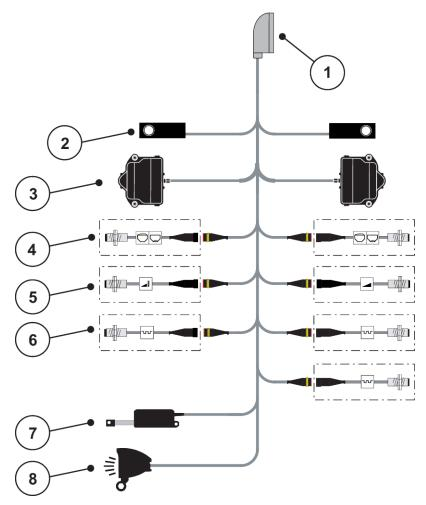
Fig. 13: Schematic connection diagram of QUANTRON-A – AXIS-M EMC V8
