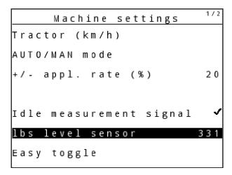
Fig. 31: Machine settings menu (example)
