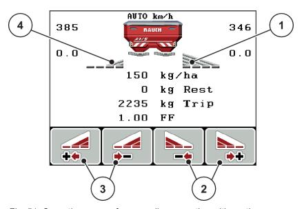
Fig. 51: Operating screen for spreading operation with sections
