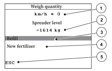
Fig. 20: Weighing the quantity menu
