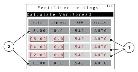
Fig. 30: VariSpread calculation, example with 8 sections (4 on each side)
