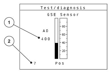
Fig. 45: Test/diagnosis; example: GSE sensor
