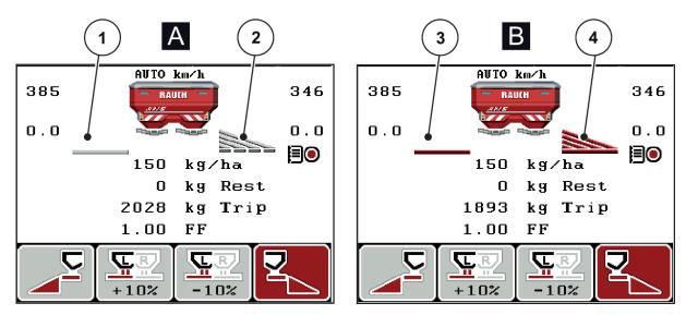
Fig. 6: Display of the AXIS metering slide status
