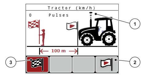
Fig. 34: Calibration run speed signal operating screen
