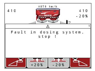
Fig. 59: Example of an alarm message
