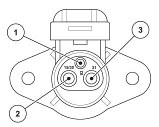
Fig. 9: PIN assignment of power socket
