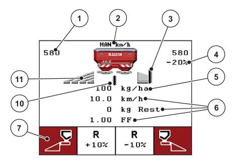
Fig. 3: Control unit display - example AXIS-M operating screen
