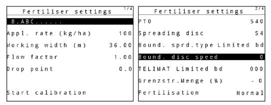
Fig. 24: Fertiliser settings menu for AXIS, Expert mode
