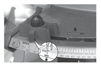
Fig. 15: AXIS metering slide preparation (example)
