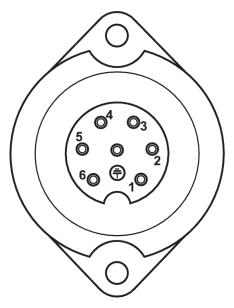
Fig. 10: PIN assignment of the 7-pin plug connector
