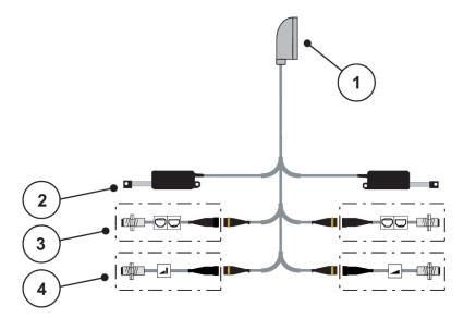
Fig. 11: Schematic connection diagram of QUANTRON-A - MDS
