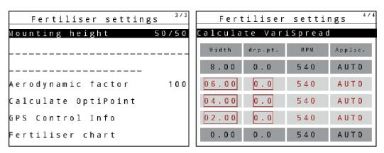
Fig. 26: Fertiliser settings menu for AXIS/MDS, tabs 3/4
