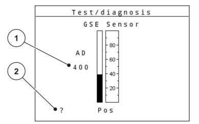
Figure 4.29: Test/diagnosis; example: Linbus
