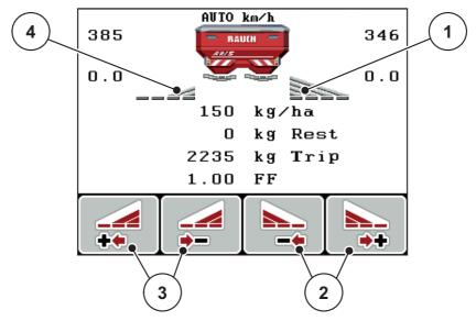
Figure 5.1: Operating screen for spreading operation with sections
