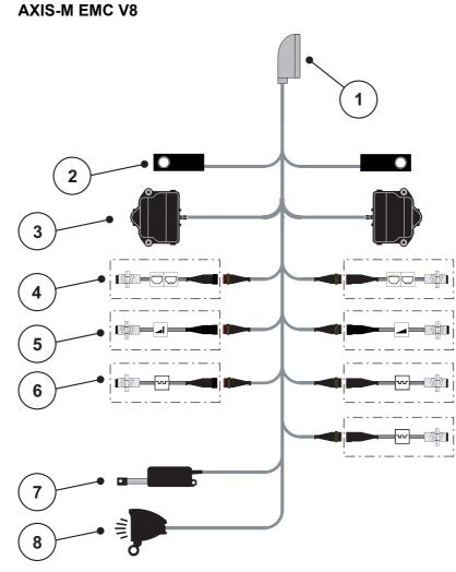
Figure 3.8: Schematic connection diagram QUANTRON-A
