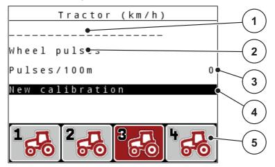
Figure 4.16: Tractor calibration menu
