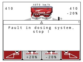
Figure 6.1: Alarm message (e.g. metering device)
