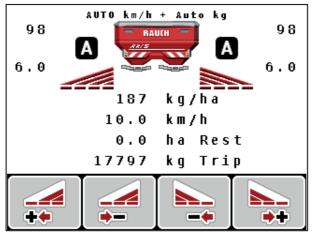
**Figure 5.6:** Spreading operation display on the operating screen with GPS Control
