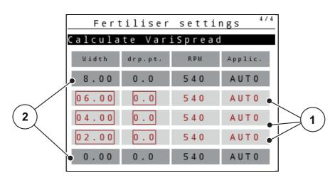
Figure 4.14: VariSpread calculation, example with 8 sections (4 on each side)
