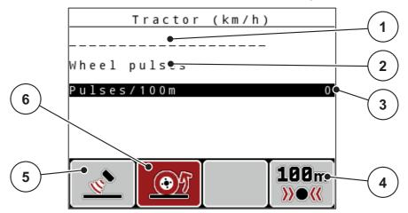
Figure 4.17: Tractor (km/h) calibration menu
