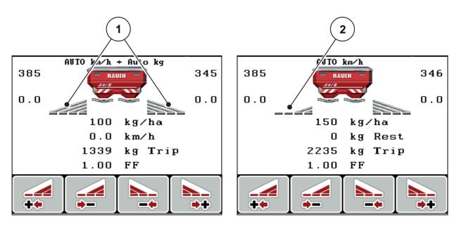
Figure 2.8: Display of the section status (example with AXIS VariSpread 8)
