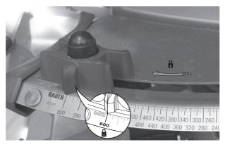
Figure 3.10: Preparing the AXIS metering slide (example)
