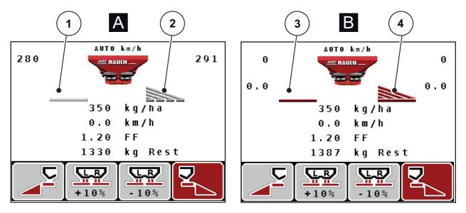
Figure 2.7: MDS metering slide status display
