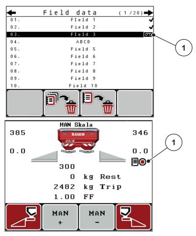
Figure 4.23: Recording symbol display
