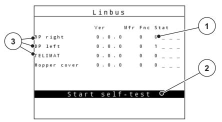
Figure 4.28: Test/diagnosis; example: Linbus
