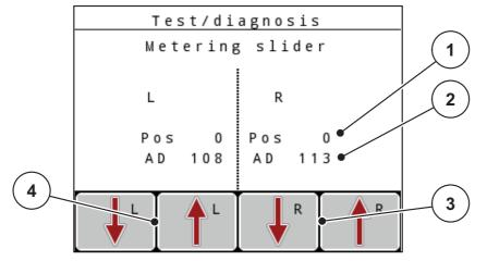
Figure 4.27: Test/diagnosis; example: Metering slide
