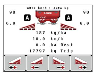
**Figure 5.6:** Spreading operation display on the operating screen with GPS Control
