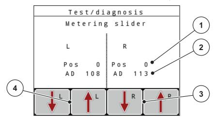
Figure 4.27: Test/diagnosis; example: Metering slide
