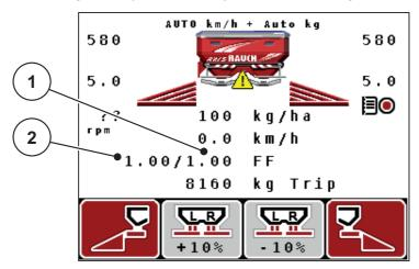
Figure 4.11: The left and right flow factors are controlled separately (M EMC function activated).
