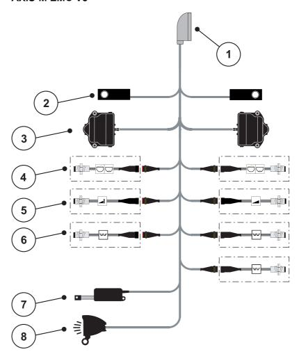
Figure 3.8: Schematic connection diagram QUANTRON-A
