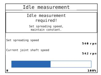
Figure 5.4: Idle measurement information screen
