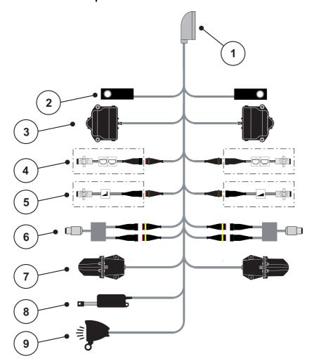
Figure 3.9: Schematic connection diagram QUANTRON-A
