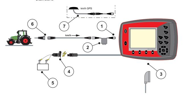
Figure 3.3: Schematic connection diagram QUANTRON-A (standard)
