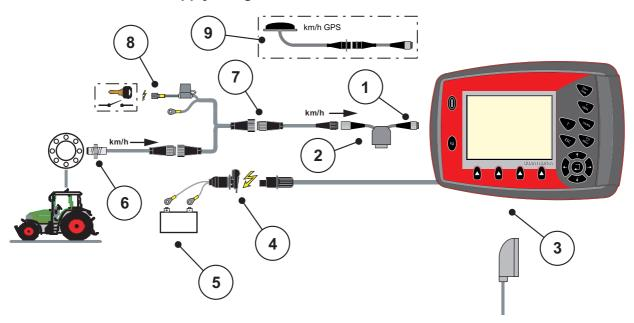
Figure 3.5: Schematic connection diagram QUANTRON-A (power supply via ignition lock)
