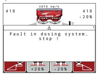
Figure 6.1: Alarm message (e.g. metering device)
