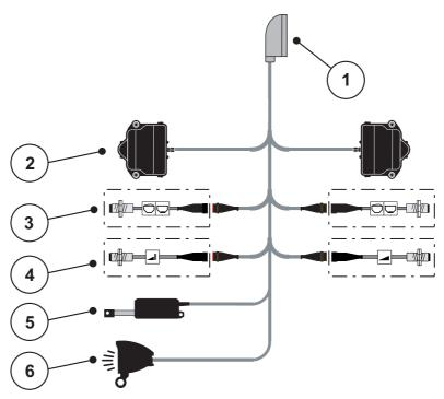
Figure 3.7: Schematic connection diagram QUANTRON-A
