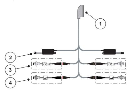
Figure 3.6: Schematic connection diagram QUANTRON-A
