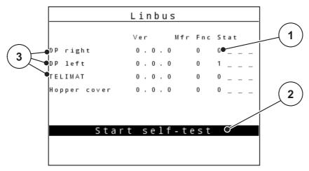
**Figure 4.28:** Test/diagnosis; example: Linbus
