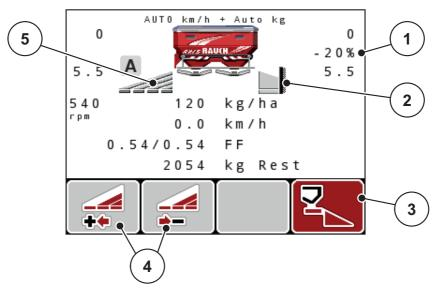
**Figure 5.3:** Operating screen, one section on the left, boundary spreading side on the right
