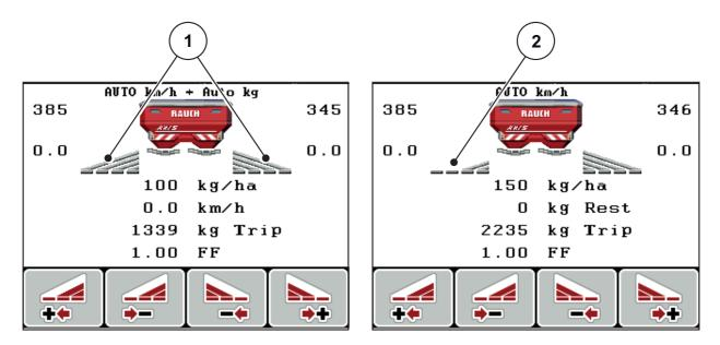
Figure 2.8: Display of the section status (example with AXIS VariSpread 8)
