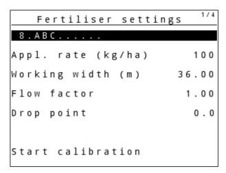
Figure 4.6: AXIS fertiliser settings menu, Easy mode
