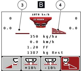
Figure 2.7: MDS metering slide status display
