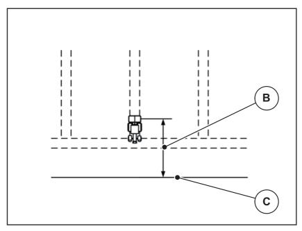
**Figure 5.8:** Switch-off distance (relating to field border)
