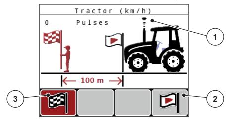
Figure 4.18: Calibration run speed signal operating screen
