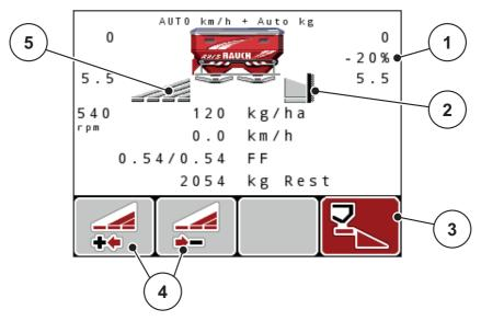
Figure 5.2: Operating screen, one section on the left, boundary spreading side on the right
