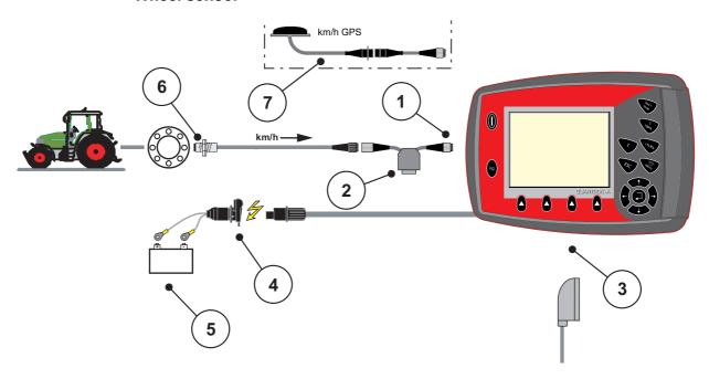
**Figure 3.4:** Schematic connection diagram QUANTRON-A (wheel sensor)
