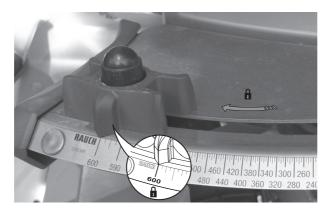
**Figure 3.10:** Preparing the AXIS metering slide (example)
