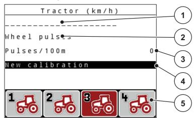
Figure 4.16: Tractor calibration menu
