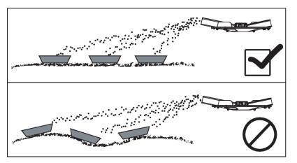
Fig. 2: Positioning the collecting vessels
