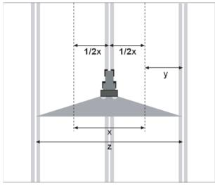
Fig. 3: Triangular spreading pattern
