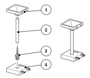
Fig. 1: Assembling measuring tubes
