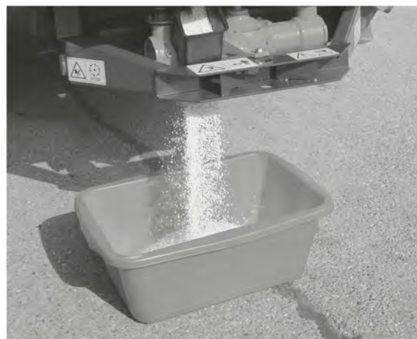
Fig. 39: Implementing the calibration test
