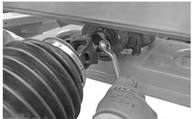
Fig. 15: Connecting the universal drive shaft
