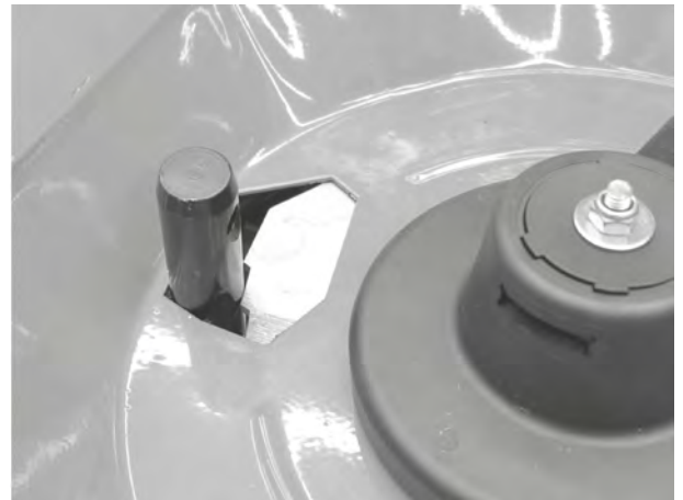
Fig. 66: Lower link pin in metering opening
