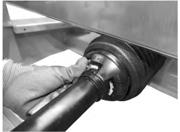
Fig. 17: Securing the universal drive shaft cover
