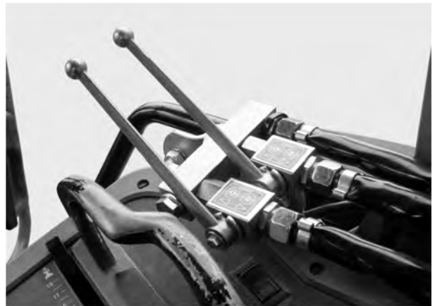
Fig. 30: Metering slide actuator of the two-way unit
