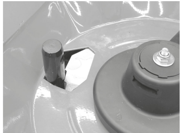
Fig. 70: Lower link pin in metering opening
