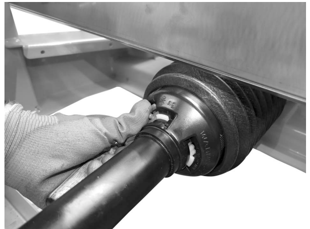
Fig. 17: Securing the universal drive shaft cover
