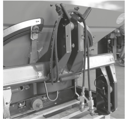
Fig. 64: Storage of the drive shaft, storage of the cables and hydraulic hoses
