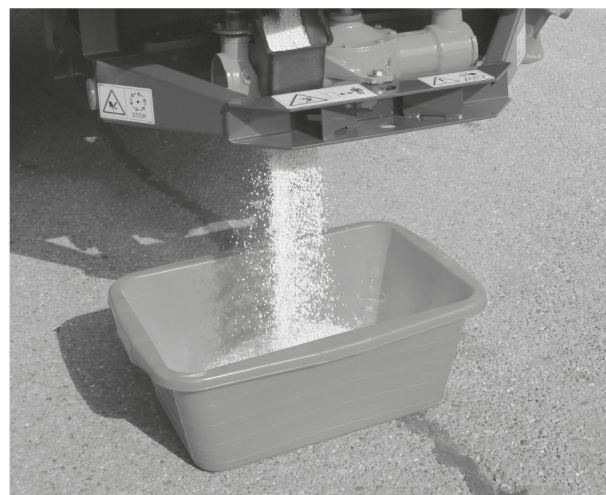
Fig. 39: Implementing the calibration test
