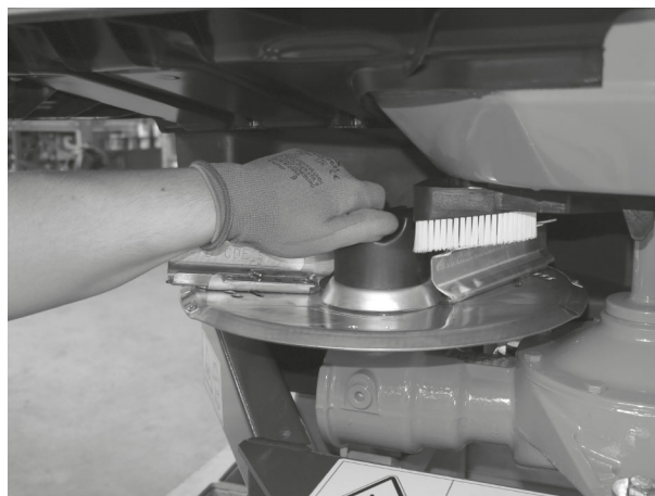
Fig. 40: Screw the cap nut on
