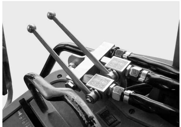
Fig. 30: Metering slide actuator of the two-way unit
