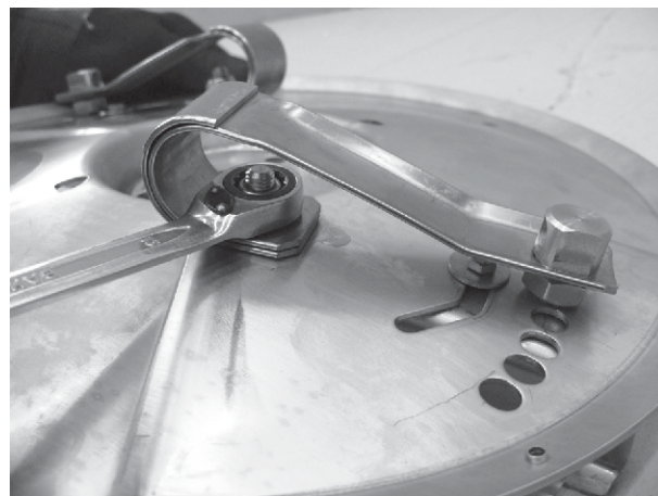
Fig. 96: Attachment of the flat spring
