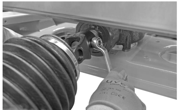
Fig. 15: Connecting the universal drive shaft
