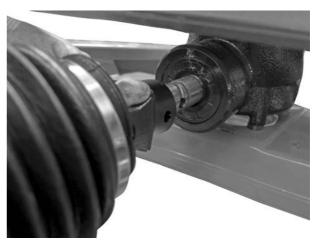
**Figure 7.2:** Push the universal drive shaft onto the transmission spigot
