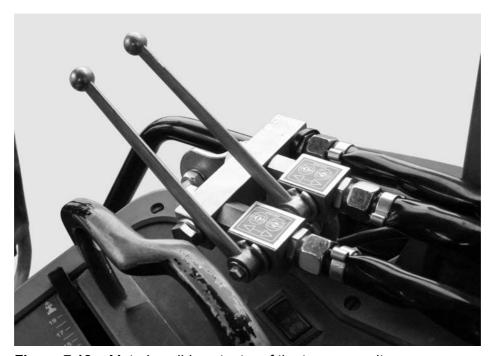
Figure 7.12: Metering slide actuator of the two-way unit
