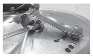
**8.** Fasten the flat spring with a new washer and a new self-locking spring fastening nut.
