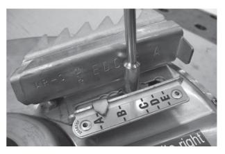
**Figure 12.27:** Spreading vane on the spreading disc
