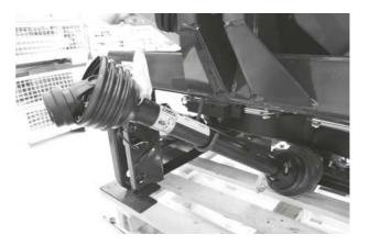
**Figure 7.6:** Retainer of the universal drive shaft
