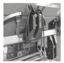
Figure 7.14: Storage of drive shaft and of hydraulic hoses
