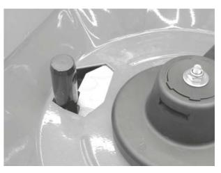
Figure 12.5: Lower link pin in metering opening
