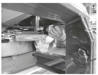
only versions K/R: Unhook the spring using the adjustment lever.
