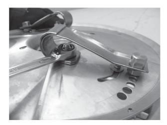
Figure 12.22: Remove the screws
