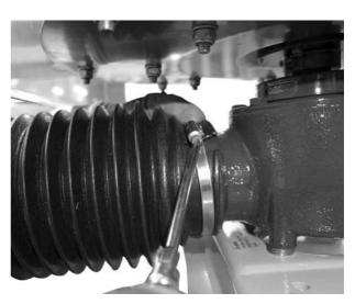
**Figure 7.4:** Mount the universal drive shaft guard
