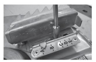
Tighten the screw so that this lies flat and tight (tightening torque: approx. 8 Nm).
