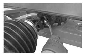
7. Tighten the hex cap screw and nut using a size 17 wrench (max. 35 Nm).
