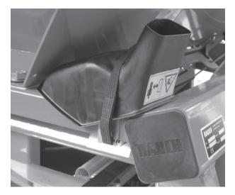
Figure 8.3: Calibration test chute
