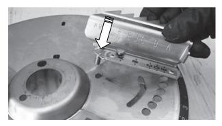
**1.** Place the new main vane on the spreading disc.
