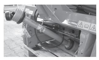
Figure 6.24: Universal drive shaft retainer
