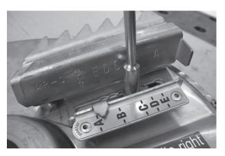
Figure 9.27: Spreader van on the spreading disc
