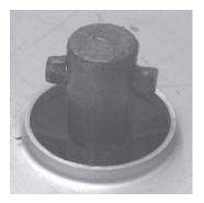
Figure 6.5: Agitator shaft
