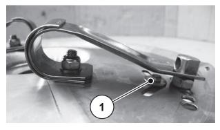
Figure 9.16: Flat spring on the spreading disc
