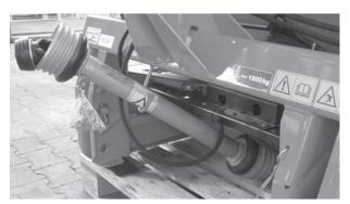
Figure 6.34: Parking the universal drive shaft and the hydraulic hoses
