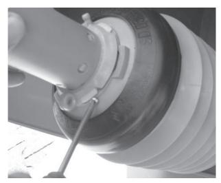
Figure 6.22: Drive shaft shield
