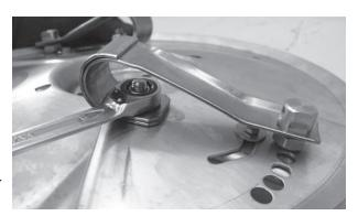
**8.** Fix the flat spring with a new washer and a new self-locking spring fixing nut.
