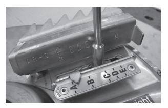
3. Tighten the bolt so that it is flat and tight (tightening torque: approx. 8 Nm).
