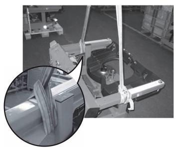
Figure 6.1: Lifting the frame
