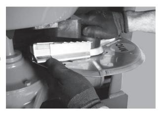
Figure 8.9: Screw on cap nuts
