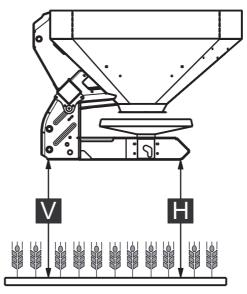
**Figure 6.12**: Maximum approved hopper height F and R in normal and late top dressing
