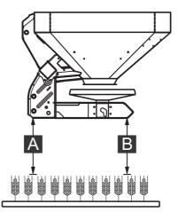
**Figure 6.13**: Hopper height A and B as per spreading charts in normal dressing
