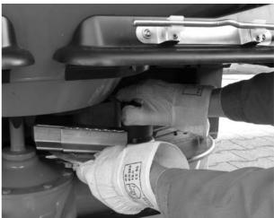
Figure 7.7: Screw on cap nuts
