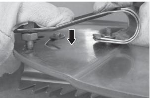
6 Carefully push the locking pin (c) into one of the positioning holes
