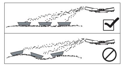
Figure 6.16: Layout of the catch trays
