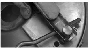
2 Remove the flat spring using a suitable screwdriver or the setting lever.
