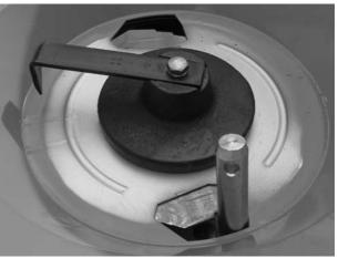
Figure 8.8: Lower link pin in outlet
