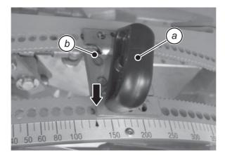
Figure 6.2: Metering slide setting to 130
