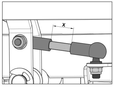
Figure 5.23: Adjusting the angle joint
