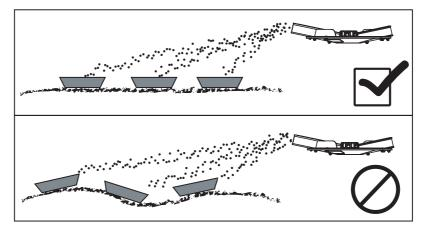
Figure 6.19: Layout of the catch trays
