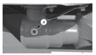
a Oil level checking screw
