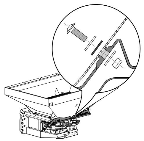
Figure 5.15: Fixing the deflection and protection device
