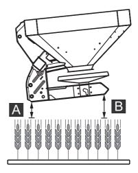
**Figure 6.14**: Hopper height A and B as per calibration charts in late top dressing
