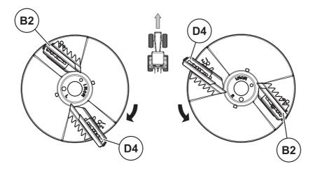
Figure 6.9: Vane adjustment, example D4-B2
