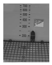
Figure 9.1: Fill level scale (graduated in litres)
