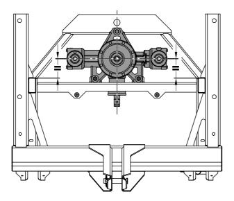
Figure 8.14: Check the location of the gearbox
