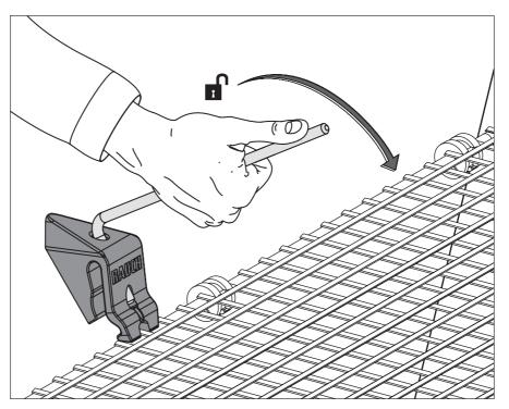
Figure 8.3: Open the safety mesh guard interlock
