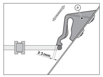
Figure 5.14: Test dimension for functional check of the safety mesh guard interlock
