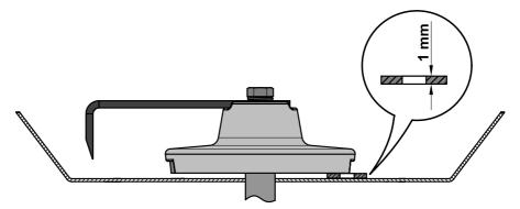
Figure 8.15: Setting the agitator
