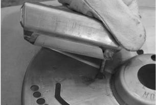
1 Place the new main vane on the spreading disc.
