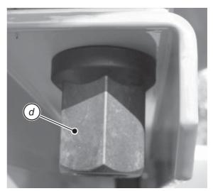
d Plastic nut, tightening torque: **90 Nm**
