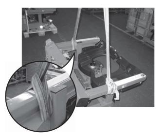
Figure 5.1: Lifting the frame
