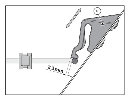
Figure 8.4: Test dimension for functional check of the safety mesh guard interlock
