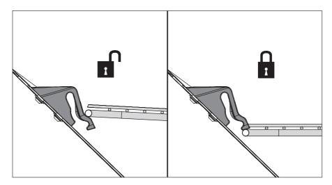
Figure 8.2: Safety mesh guard interlock open/closed
