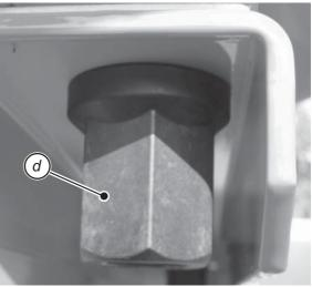
d Plastic nut, tightening torque: **90 Nm**
