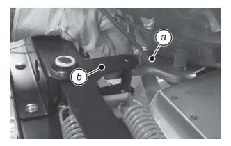
Figure 8.6: Pull the metering slide to the stop
