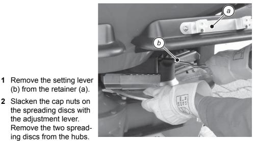
Figure 8.11: Slackening cap nuts
