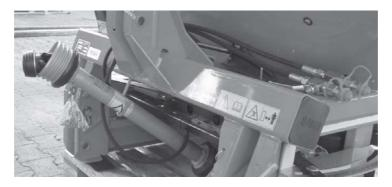
Figure 5.25: Parking the universal drive shaft and the hydraulic hoses
