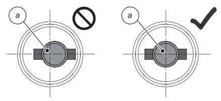
Figure 8.13: Centring the drive spigot
