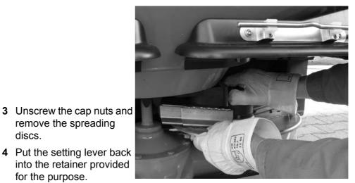
Figure 8.12: Unscrewing cap nuts
