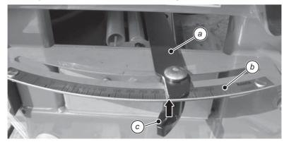
**Figure 6.3**: Scale for setting the spreading volume (on the left hand side looking in the direction of travel)
