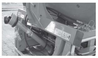
Figure 5.20: Universal drive shaft retainer
