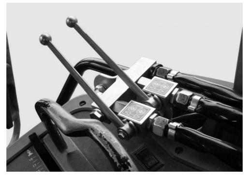
Figure 5.21: Slide actuator of the two-way unit
