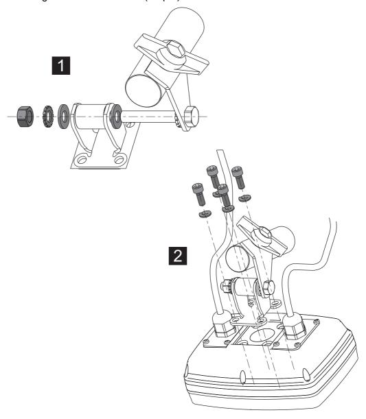
Figure 3.2: Installing the unit holder
