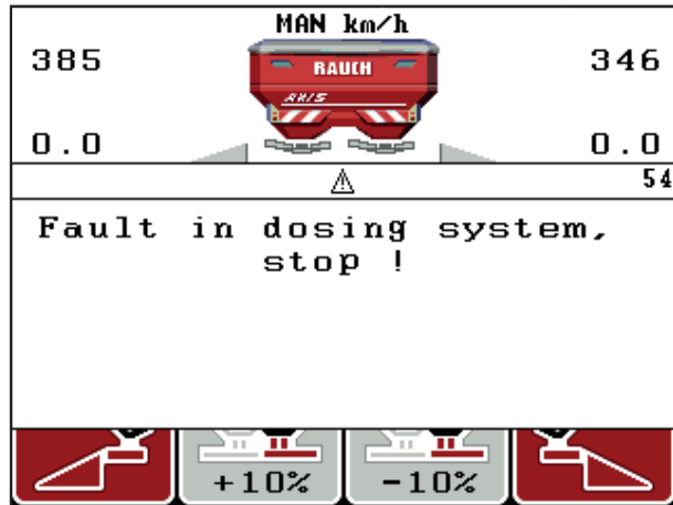
Figure 6.1: Alarm message (e.g. metering device)
