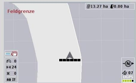
The headland is plotted in light grey, the sections are automatically switched off in this area.
