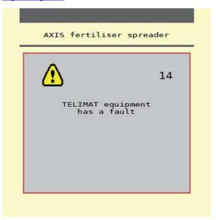
Figure 5.2: TELIMAT alarm message display
