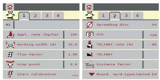
Figure 4.11: Fertiliser settings menu, tab 1 and 2
