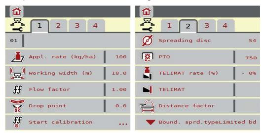
Figure 4.2: Fertiliser settings menu, tab 1 and 2
