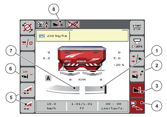
Fig. 43: Operating screen with one section on the left, border spreading side on the right
