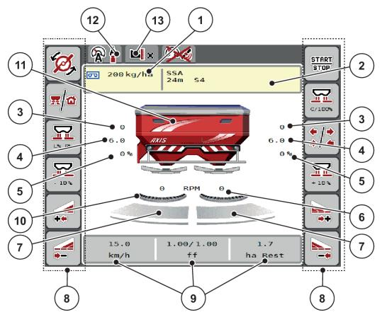
Fig. 1: Machine control unit display
