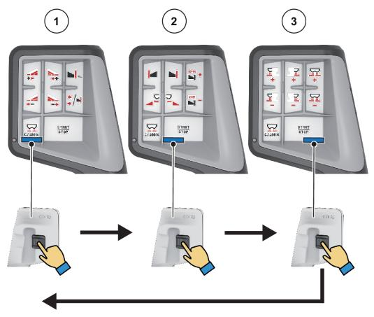
Fig. 32: CCI A3 joystick, operating level display
