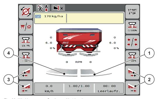
Fig. 39: Working screen: Sections with 4 levels
