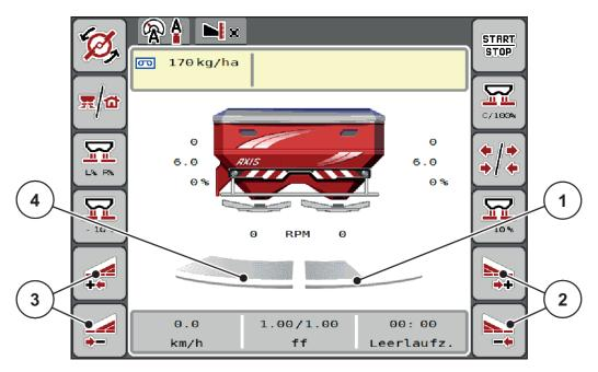
Fig. 41: Working screen: Continuous section control
