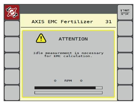
Fig. 44: Alarm display of idle measurement
