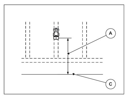
Fig. 48: Distance on (measured from field border)
