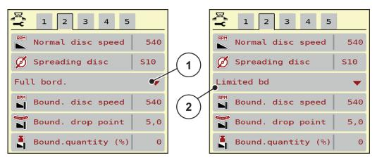
Fig. 14: Limited border spreading mode setting values
