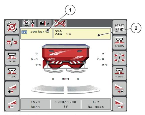
Fig. 13: Entering the application rate on the touch screen
