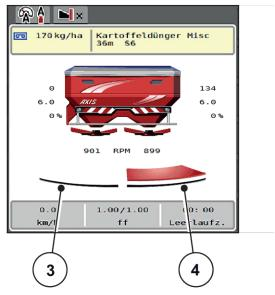
Fig. 4: Display of the metering slide status
