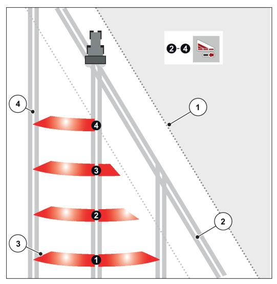
Fig. 40: Automatic section control
