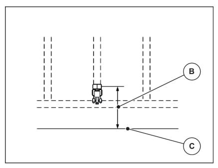
Fig. 49: Distance off (measured from field border)
