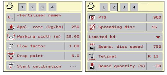
Fig. 11: Fertiliser settings menu AXIS-M, tabs 1 and 2
