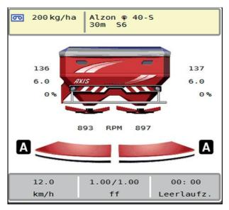
**Figure 5.11:** Spreading operation display on the operating screen with GPS Control
