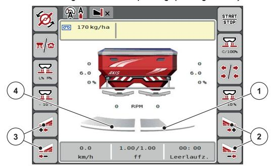
Figure 5.5: Operating screen, 2 section widths
