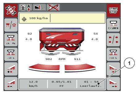
**Figure 5.9:** Display of the idle measurement on the operating screen
