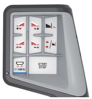
Figure 4.23: Key assignment level 1
