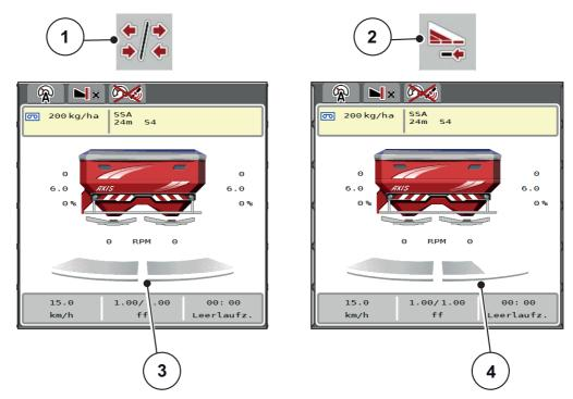
Figure 2.5: Display of the section status
