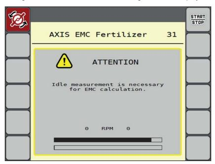
During the idle measurement, the following window is displayed.
