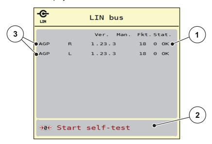
Figure 4.15: Test/diagnosis; example: Linbus
