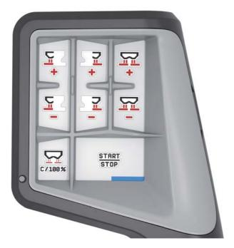
Figure 4.25: Key assignment level 3
