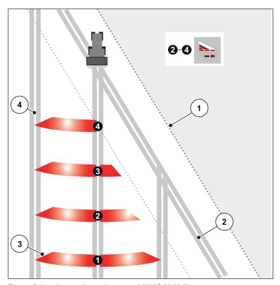
Figure 5.4: Automatic section control (AXIS-M 20.2)
