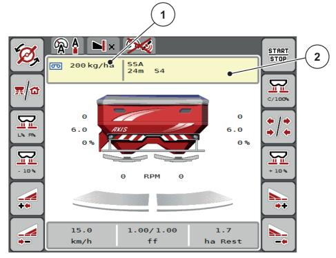
Figure 4.9: Managing the fertiliser chart via the touch screen
