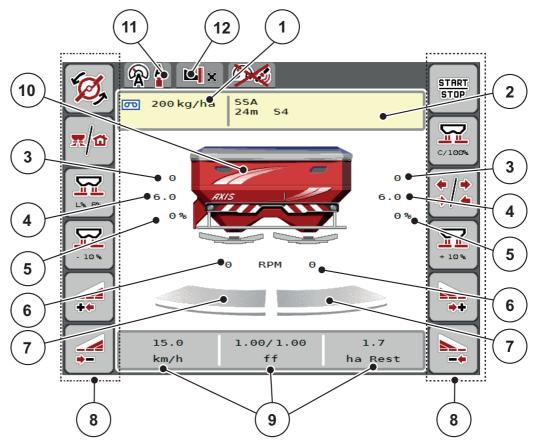
Figure 2.1: Machine control unit display
