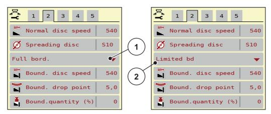
Figure 4.6: Limited boundary spreading mode setting values
