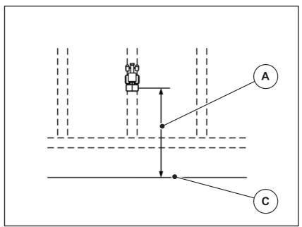
**Figure 5.12:** Switch-on distance (relating to field border)
