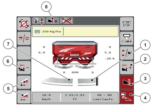
**Figure 5.7:** Operating screen, one section on the left, limited border spreading side on the right
