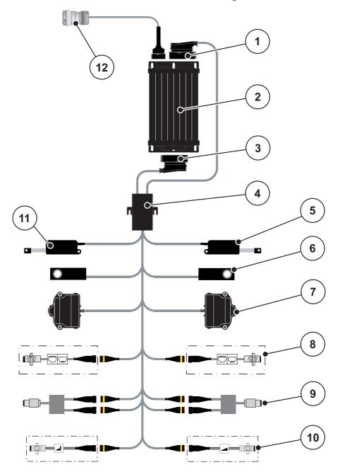
AXIS-M 20.2 EMC: Schematic connection diagram
