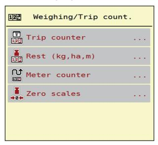
Figure 4.16: Weighing trip counter menu
