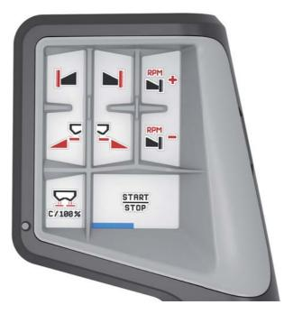
Figure 4.24: Key assignment level 2
