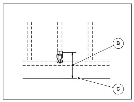
**Figure 5.13:** Switch-off distance (relating to field border)
