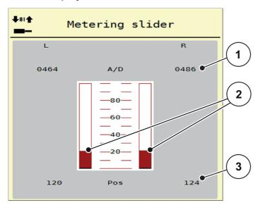
Figure 4.14: Test/diagnosis; example: Metering slide
