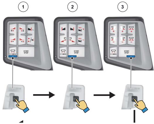
Figure 4.22: CCI A3 joystick, operating level display
