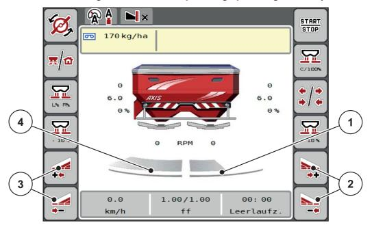
Figure 5.3: Operating screen, 2 section widths
