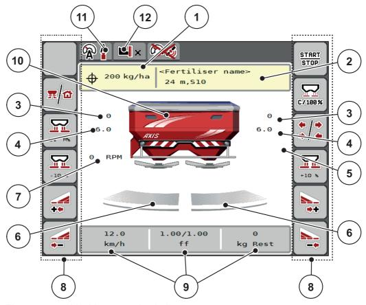
Machine control unit display Figure 2.2:
