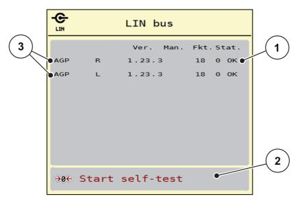
Figure 4.16: Test / Diagnosis, example: Linbus
