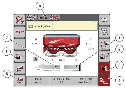
**Figure 5.5:** Operating screen, one section width on the left, limited border spreading side on the right
