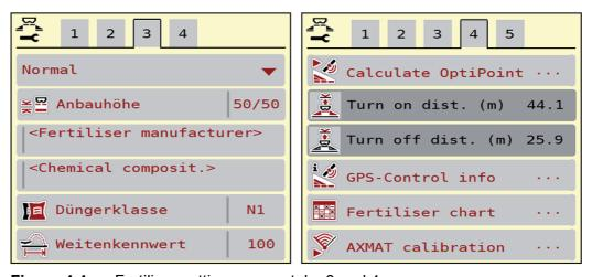
Figure 4.4: Fertiliser settings menu, tabs 3 and 4
