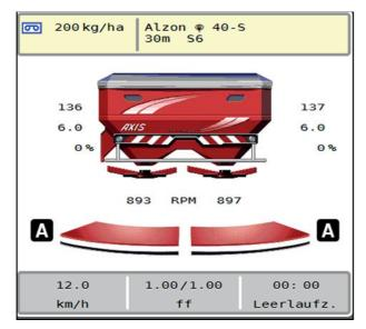
**Figure 5.9:** Spreading operation display on the operating screen with GPS Control
