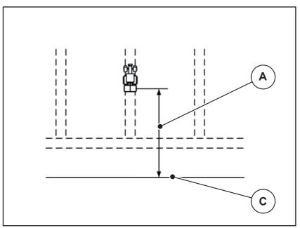
**Figure 5.10:** Switch-on distance (relating to field border)
