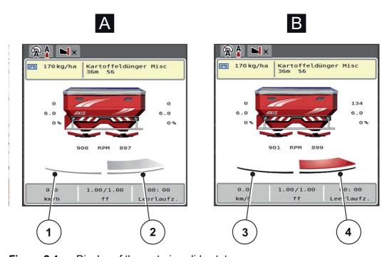
**Figure 2.4:** Display of the metering slide status
