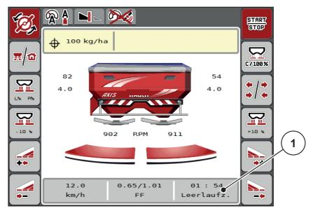
**Figure 5.7:** Display of the idle measurement on the operating screen
