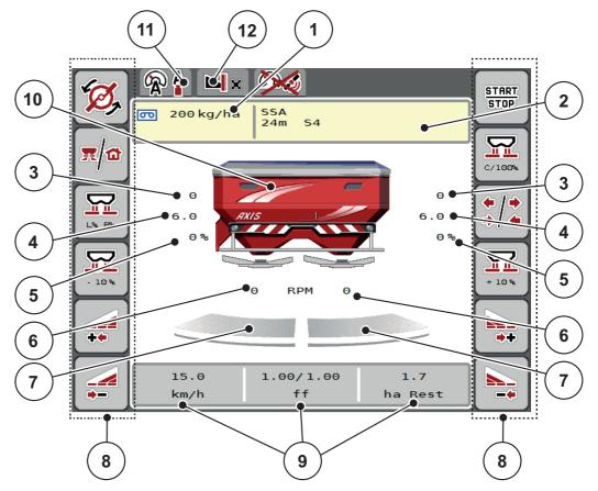
Figure 2.1: Machine control unit display
