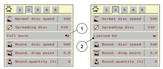
Figure 4.6: Limited border spreading mode setting values
