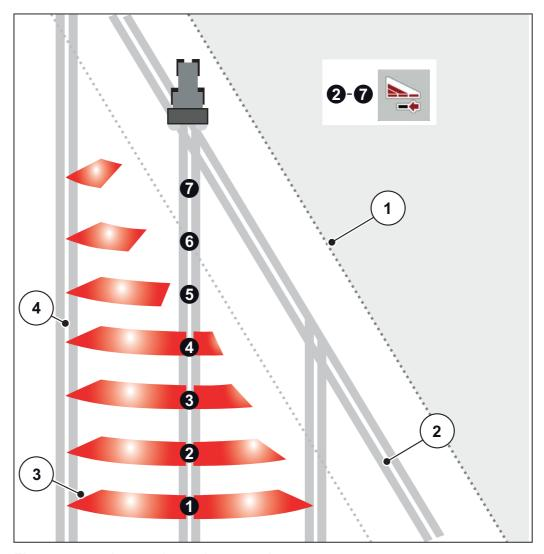
Figure 5.4: Automatic section control
