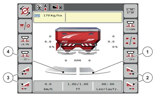
Figure 5.3: Operating screen, 2 section widths
