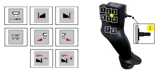
Figure 4.23: Key assignment, level 2 (LED is yellow)
