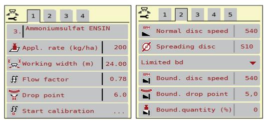
Figure 4.2: Fertiliser settings menu AXIS-H, tabs 1 and 2
