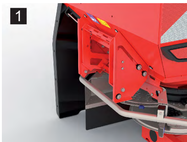
Fig. 10: Folding up the steps into the transport position
