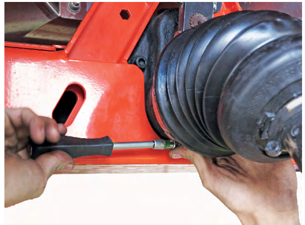
Fig. 20: Tighten the hose clamp
