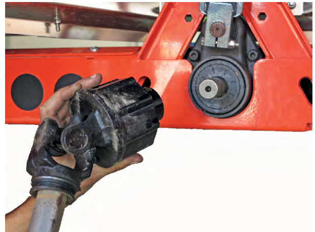
Fig. 16: Pushing the universal drive shaft on to the PTO spigot
