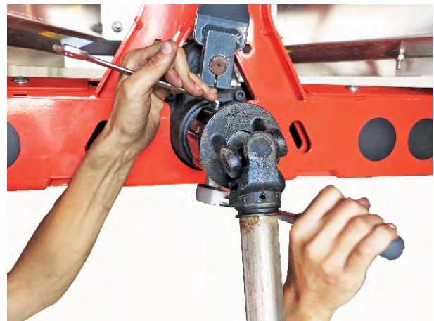
Fig. 17: Fastening the universal drive shaft
