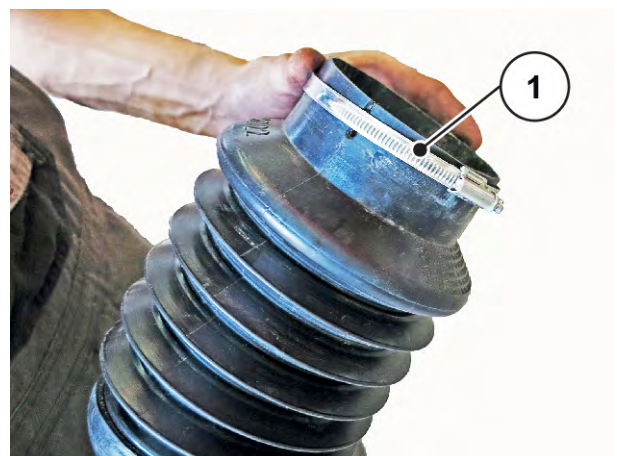
Fig. 17: Fastening the universal drive shaft
