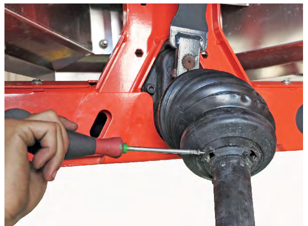
Fig. 19: Securing the universal drive shaft cover
