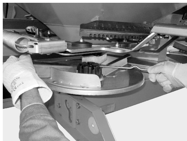
Fig. 38: Loosening the cap nut
