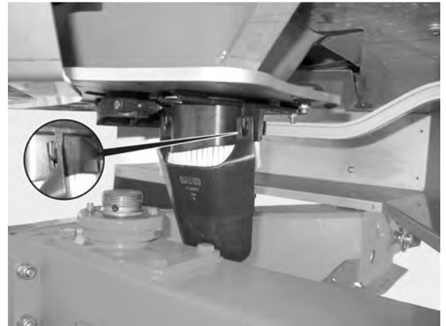
Fig. 38: Attaching the calibration test chute
