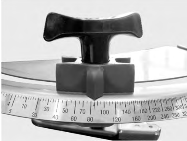
Fig. 62: Metering slide adjustment scale
