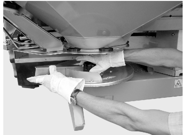
Fig. 46: Tighten the cap nut
