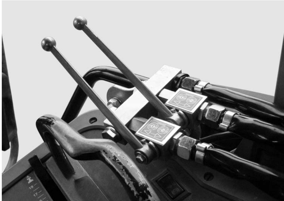
Figure 7.8: Slide actuator of the two-way unit
