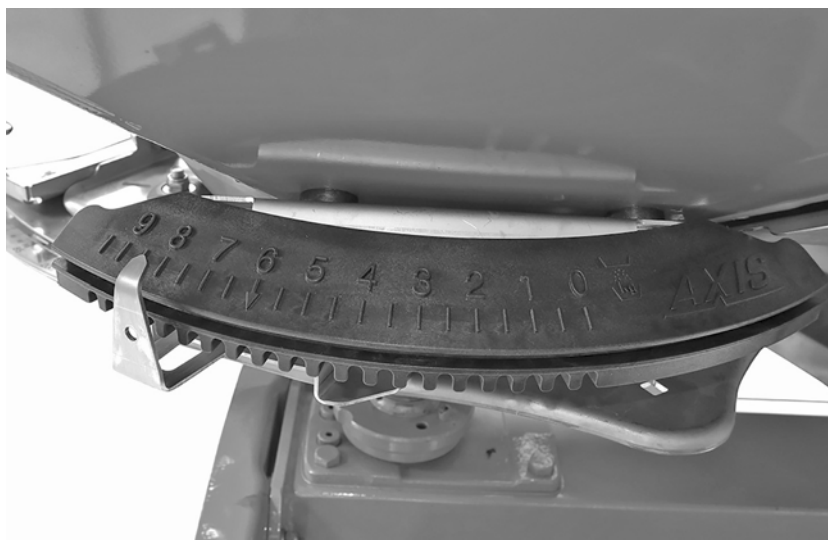
Figure 8.6: Drop point display (example)
