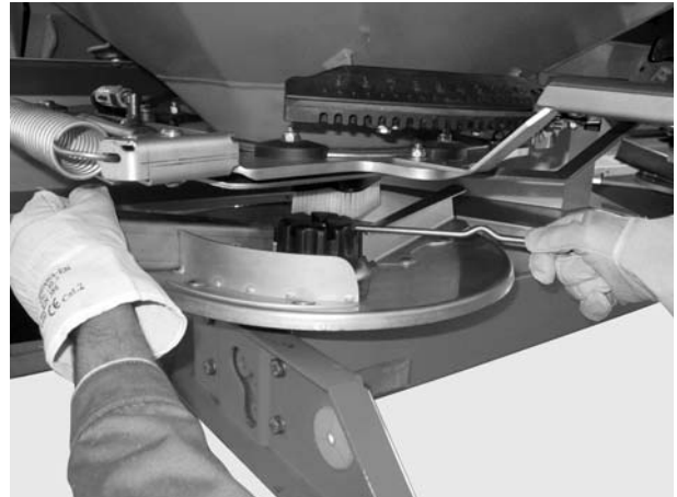
Figure 8.13: Loosen cap nut
