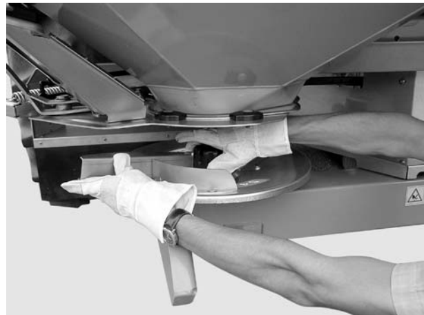
Figure 8.16: Screw on the cap nut
