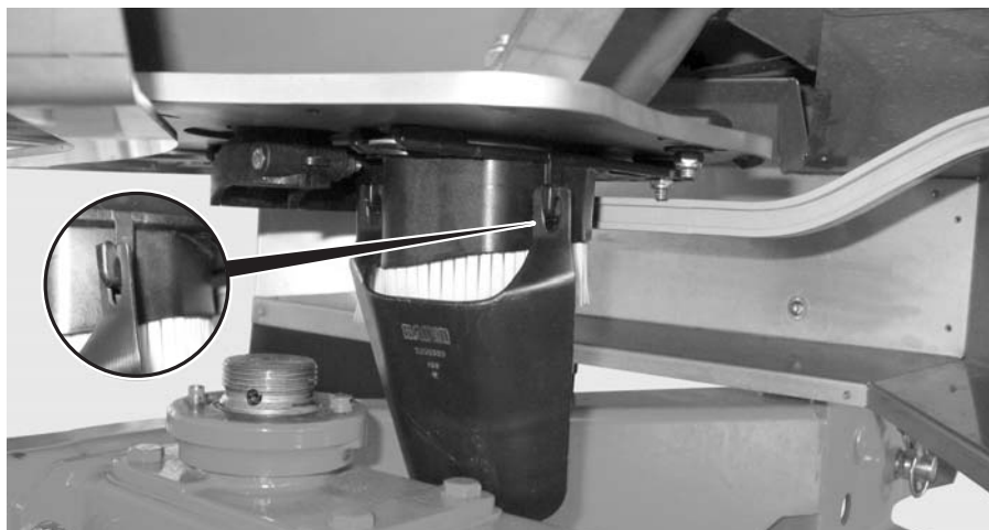
Figure 8.14: Attach the calibration test chute
