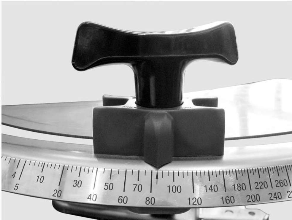
Figure 10.19: Adjustment scale of metering slide
