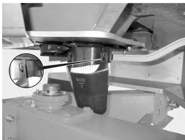
Fig. 49: Attaching the calibration test chute
