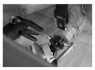
Fig. 13: Fastening the universal drive shaft
