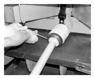
Fig. 16: Securing the universal drive shaft cover
