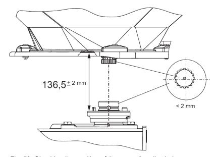
Fig. 59: Checking the position of the spreading disc hub
