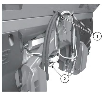
Fig. 21: Storage of the cables and hydraulic hoses
