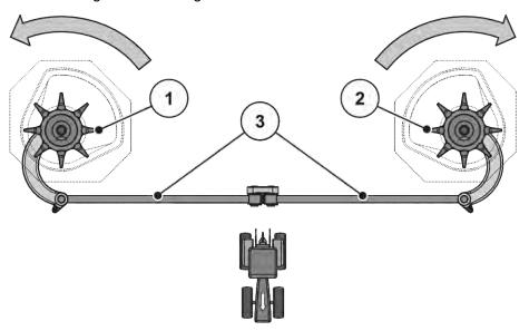
Fig. 60: Checking the agitator drive
