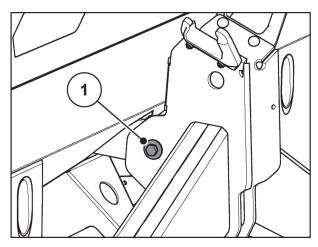
Fig. 53: Fastening the tie rod at the weigh frame
