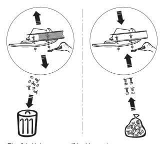
Fig. 64: Using new self-locking nuts
