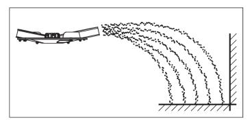
Fig. 28: Limited border spreading during normal fertilizing
