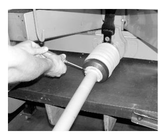
Fig. 20: Securing the universal drive shaft cover
