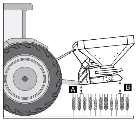
Fig. 26: Attachment of the machine on the lower coupling point of the lower link
