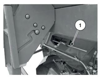
Fig. 36: Position of the adjustment lever AXIS xx.2
