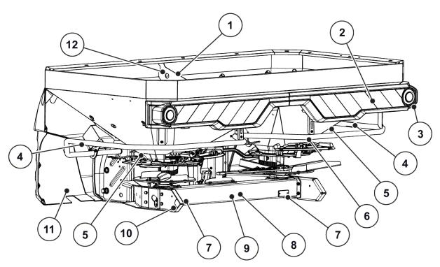
Fig. 3: Safety equipment, warning and instruction stickers, rear
