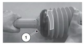
Fig. 10: Loosening the universal drive shaft guard
