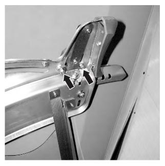
Fig. 70: Release the adjustment sheet from the discharge point
