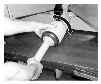
Fig. 15: Attaching the universal drive shaft guard
