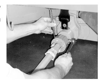
Fig. 18: Fastening the universal drive shaft
