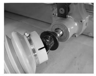
Fig. 12: Pushing the universal drive shaft on to the transmission spigot
