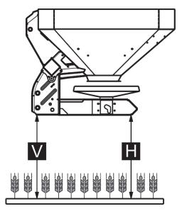
Fig. 23: Maximum admissible mounting height during normal and late fertilizing
