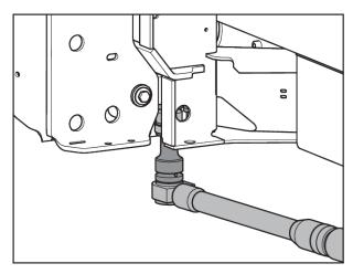
Fig. 52: Fastening the weigh cells (on the left side of the direction of travel)
