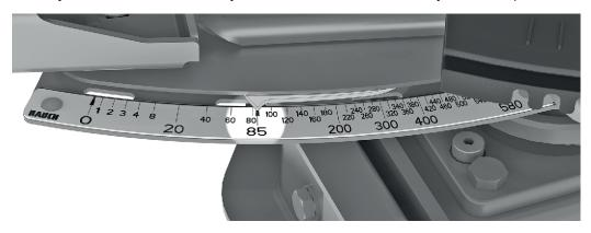
Fig. 68: Metering slide pointer on scale value 85
