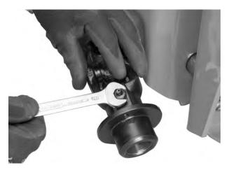
Fig. 11: Slacken the grease nipple
