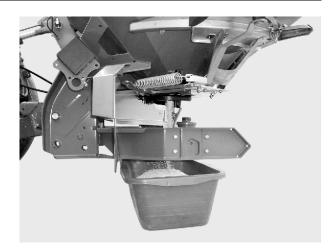
Fig. 49: Perform a calibration test
