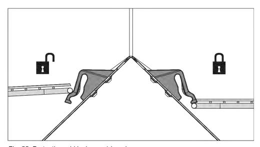
Fig. 55: Protective grid lock open/closed
