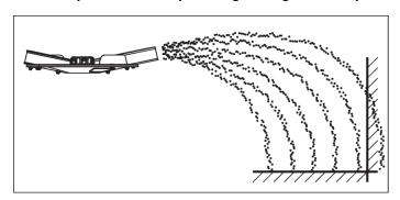
Fig. 29: Border spreading during normal fertilizing
