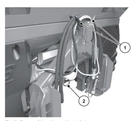
Fig. 51: Storage of the cables and hydraulic hoses
