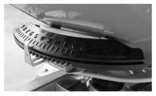
Fig. 40: Drop point display (example)
