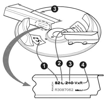
Fig. 62: Spreading disc label
