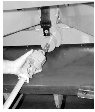
Fig. 17: Pushing the universal drive shaft on to the transmission spigot
