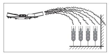
Fig. 32: Border spreading during late fertilizing
