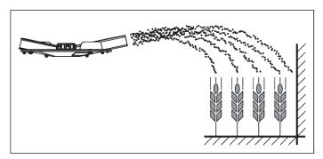
Fig. 31: Border spreading during late fertilizing
