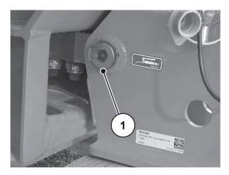
Fig. 73: Lubrication point of weighing spreaders
