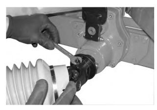
Fig. 14: Tighten the grease nipple
