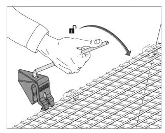
Fig. 56: Opening the protective grid lock
