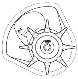
Fig. 61: Agitator head wear range
