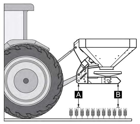
Fig. 24: Mounting position and height during normal fertilizing
