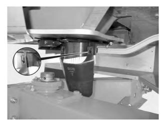
Fig. 48: Attaching the calibration test chute
