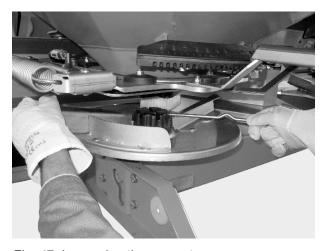
Fig. 47: Loosening the cap nut
