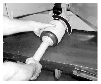
Fig. 19: Attaching the universal drive shaft guard
