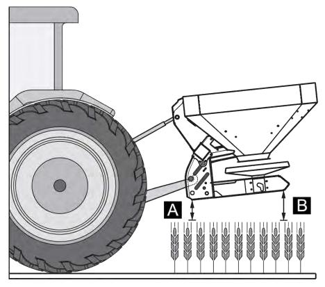
Fig. 25: Mounting position and height during late fertilizing
