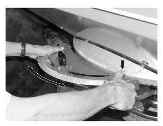
Fig. 39: Drop point adjustment center
