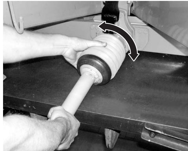
Figure 7.8: Put the universal drive shaft guard back on
