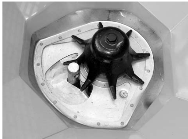
Figure 10.14: Lower link pin in metering opening
