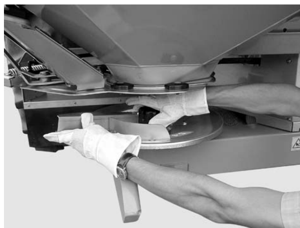
Figure 8.15: Screw on the cap nut
