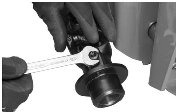
Figure 7.2: Remove lubricating nipples
