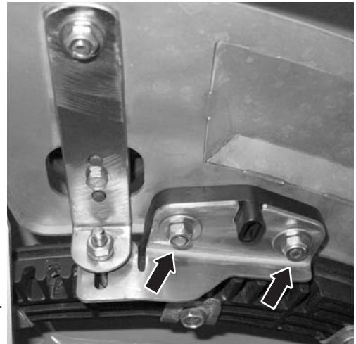
Figure 10.17: Loosen the drop point adjustment plate
