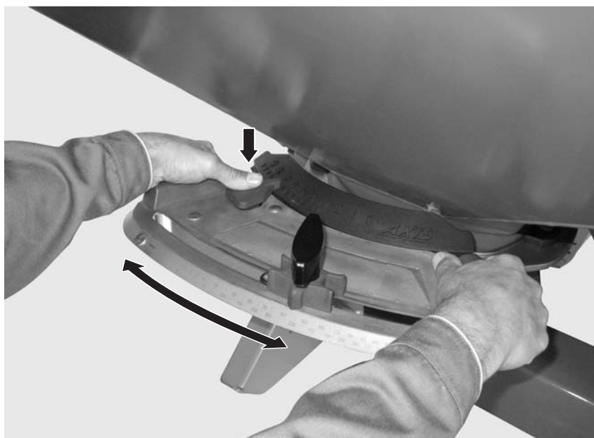
Figure 8.5: Adjustment centre for drop point
