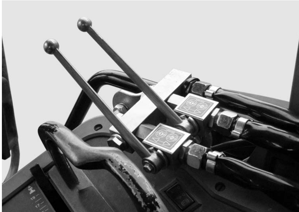
Figure 7.12: Slide actuator of the two-way unit
