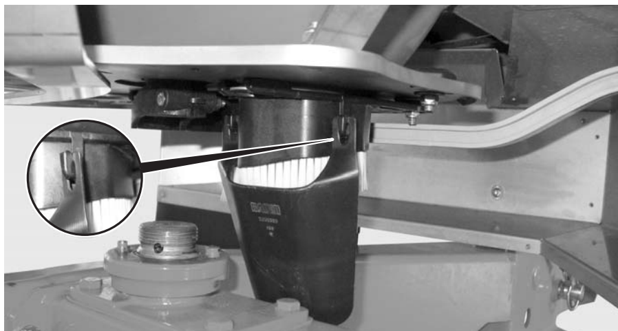
Figure 8.13: Attach the calibration test chute
