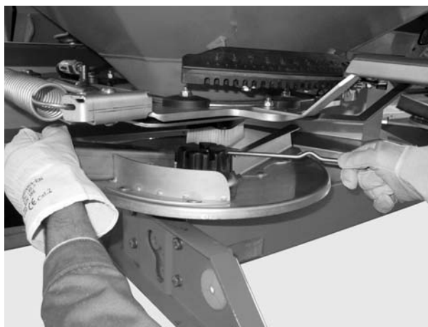
Figure 8.3: Loosen the cap nut
