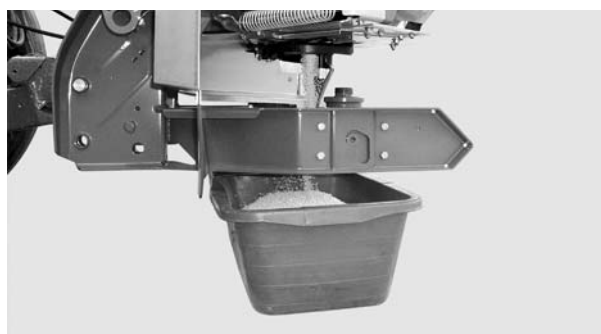
Figure 8.14: Implement the calibration test
