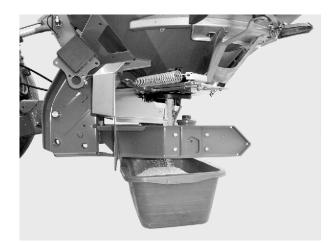
Fig. 38: Perform a calibration test
