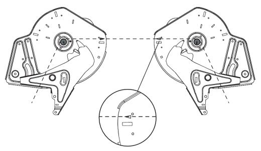
Fig. 61: Checking the drop point
