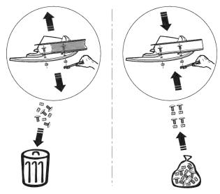
Fig. 57: Using new self-locking nuts
