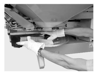
Fig. 39: Tighten the cap nut
