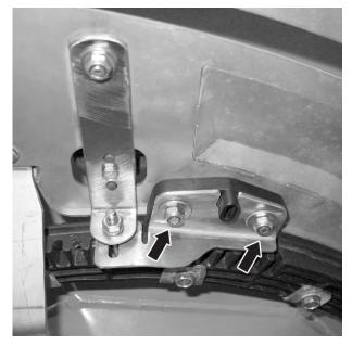
Fig. 62: Release the adjustment sheet from the discharge point
