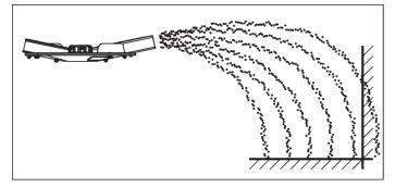
Fig. 20: Full border spreading during normal fertilizing
