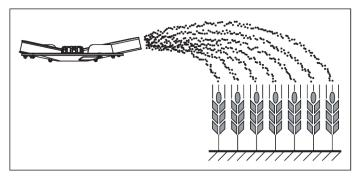
Fig. 21: Field spreading during late fertilizing
