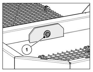
Fig. 47: Fastening the tie rod at the hopper
