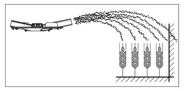
Fig. 23: Full border spreading during late fertilizing
