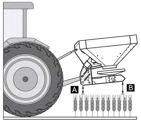
Fig. 16: Mounting position and height during late fertilizing
