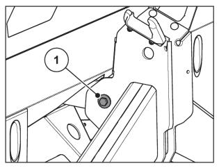
Fig. 46: Fastening the tie rod at the weigh frame
