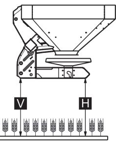
Fig. 14: Maximum admissible mounting height during normal and late fertilizing
