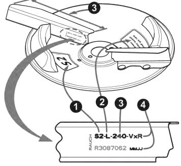
Fig. 55: Spreading disc label
