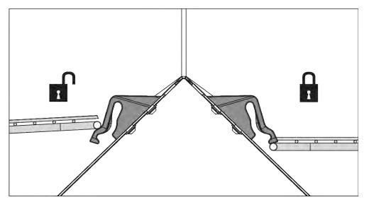
Fig. 48: Protective grid lock open/closed
