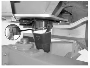
Fig. 37: Attaching the calibration test chute
