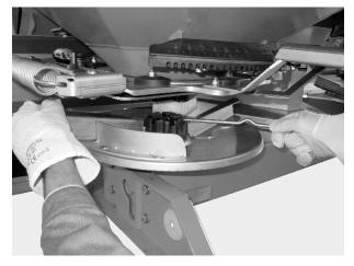
Fig. 36: Loosening the cap nut
