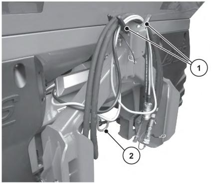
Fig. 40: Storage of the cables and hydraulic hoses
