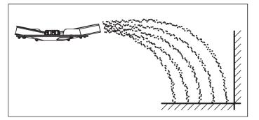
Fig. 19: Limited border spreading during normal fertilizing
