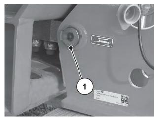
Fig. 64: Lubrication point of weighing spreaders
