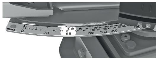
Fig. 60: Metering slide pointer on scale value 85
