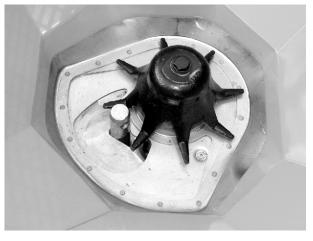
Fig. 58: Lower link pin in metering opening
