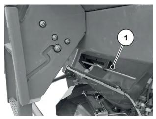
Fig. 26: Position of the adjustment lever AXIS xx.2
