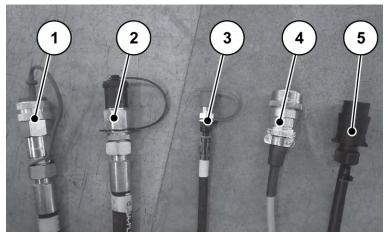
Fig. 13: Connection cables for the mineral fertilizer spreader
