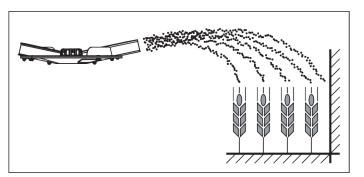
Fig. 22: Border spreading during late fertilizing
