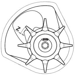
Fig. 54: Agitator head wear range
