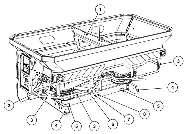
Fig. 3: Safety equipment, warning and instruction stickers, rear
