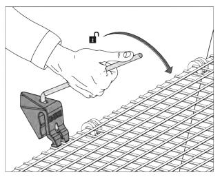
Fig. 49: Opening the protective grid lock
