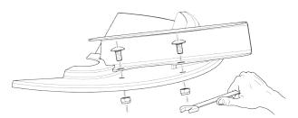
*Fig. 56: Loosening the screws of the spreading vane*
