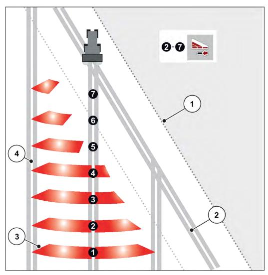
Fig. 32: Example of section connections using VariSpread pro
