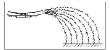
**Example of field spreading during normal spreading of fertilizer:**
