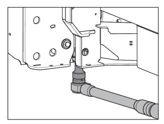
Fig. 45: Fastening the weigh cells (on the left side of the direction of travel)
