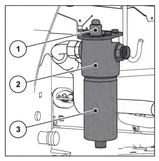
Fig. 66: Hydraulic pressure filter
