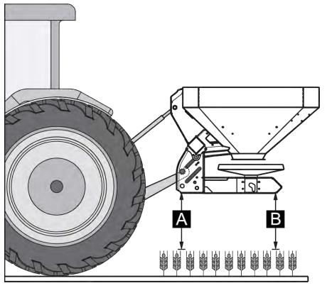
Fig. 15: Mounting position and height during normal fertilizing
