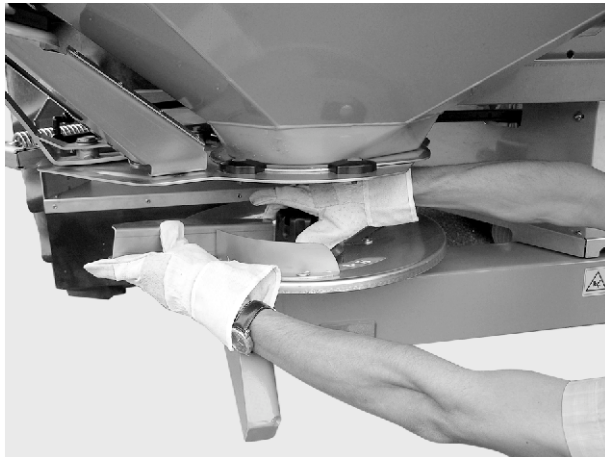
Fig. 39: Screw the cap nut on
