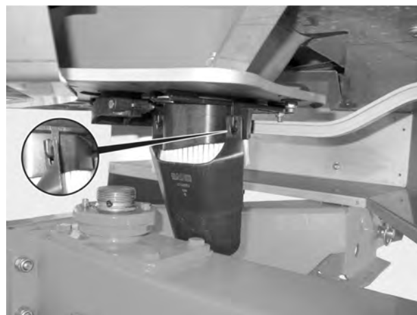
Fig. 38: Henge inn kalibreringssklike
