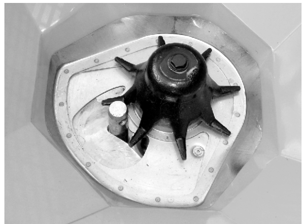
Fig. 59: Lower link pin in metering opening
