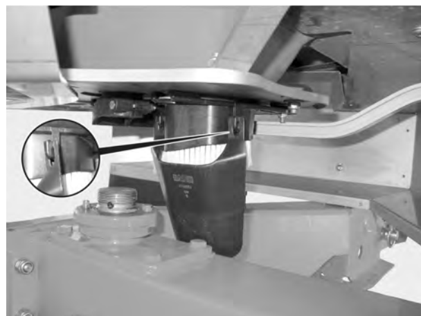
Fig. 38: Attaching the calibration test chute
