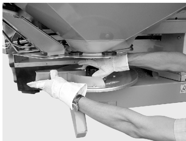
Fig. 40: Tighten the cap nut
