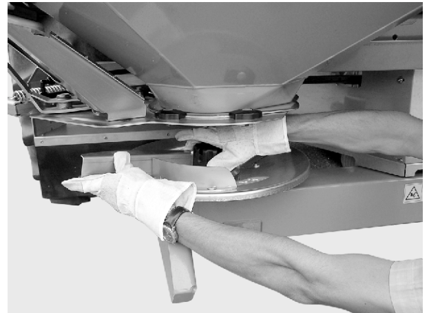
Fig. 29: Unscrew the cap nut
