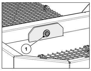
Fig. 48: Fastening the tie rod at the hopper
