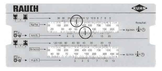
Fig. 35: Scale for calculation of the nominal output volume per minute
