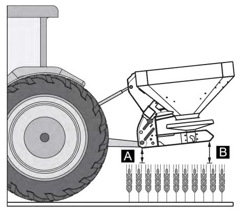
Fig. 18: Attachment of the machine on the lower coupling point of the lower link
