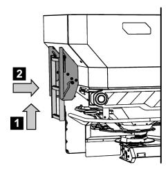
Fig. 45: Steps in the folded in position
