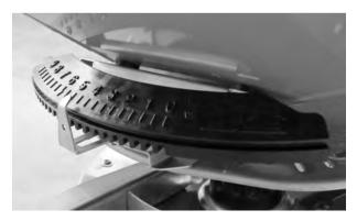
Fig. 30: Drop point display (example)
