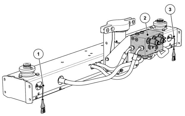
Fig. 7: Mass flow control by measuring the torque of the spreading discs
