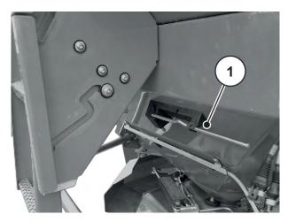
Fig. 27: Position of the adjustment lever AXIS xx.2
