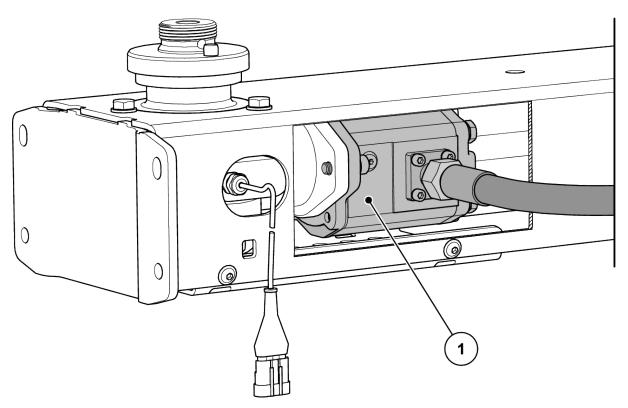
Fig. 8: Hydraulic motor for the spreading disc drive
