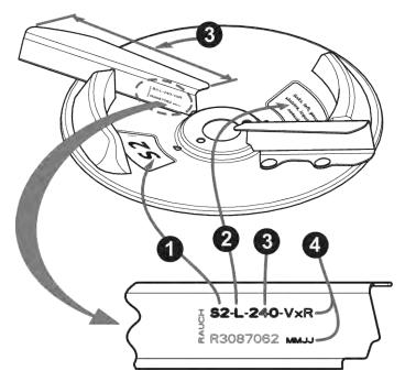
Fig. 56: Spreading disc label
