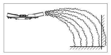
Fig. 21: Full border spreading during normal fertilizing
