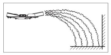
Fig. 20: Limited border spreading during normal fertilizing
