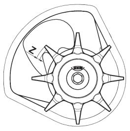
Fig. 55: Agitator head wear range
