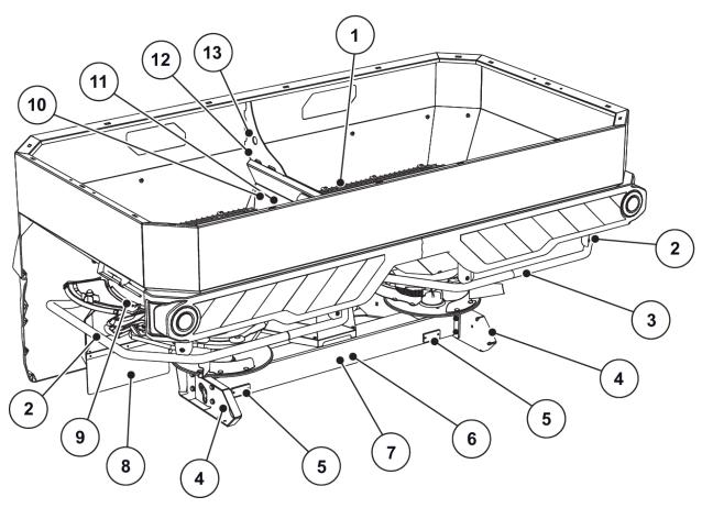
Fig. 3: Safety equipment, warning and instruction stickers, rear
