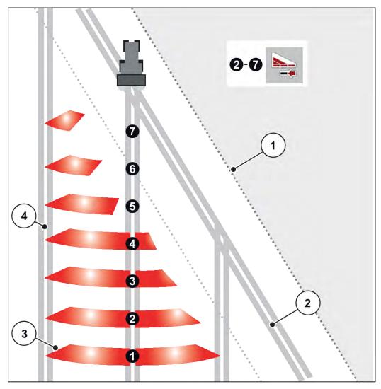
Fig. 33: Example of section connections using VariSpread pro
