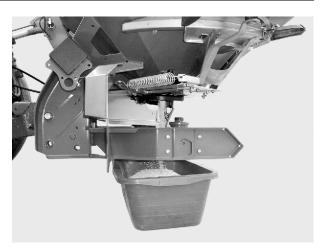
Fig. 39: Perform a calibration test
