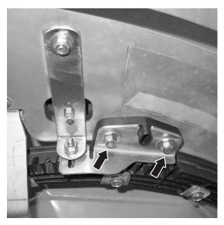
Fig. 63: Release the adjustment sheet from the discharge point
