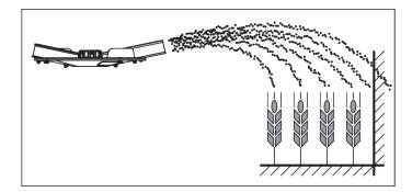
Fig. 24: Full border spreading during late fertilizing
