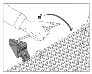
Fig. 50: Opening the protective grid lock
