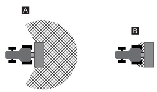
Fig. 1: Hazard zone when devices are attached
