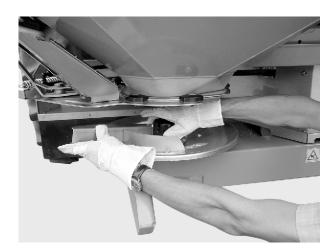
Fig. 29: Unscrew the cap nut
