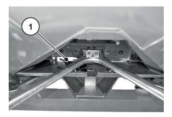
Fig. 36: Calibration test chute
