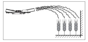
Fig. 23: Border spreading during late fertilizing
