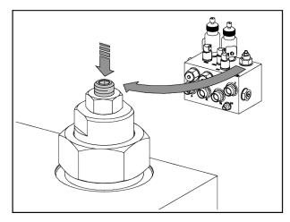
Fig. 14: For LS, adjust the adjusting screw on the hydraulic block
