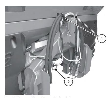
Fig. 41: Storage of the cables and hydraulic hoses
