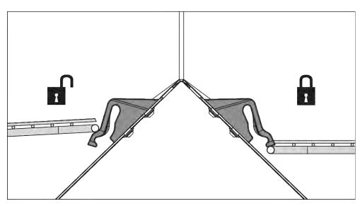
Fig. 49: Protective grid lock open/closed
