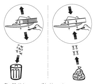
Fig. 58: Using new self-locking nuts
