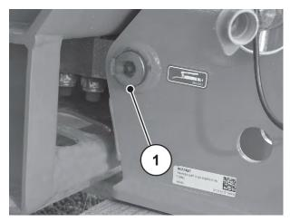
Fig. 65: Lubrication point of weighing spreaders
