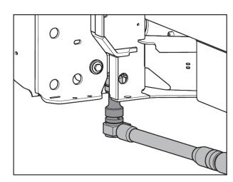
Fig. 46: Fastening the weigh cells (on the left side of the direction of travel)
