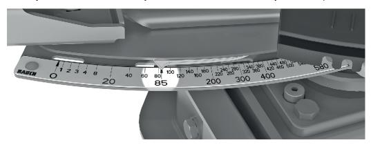
Fig. 61: Metering slide pointer on scale value 85
