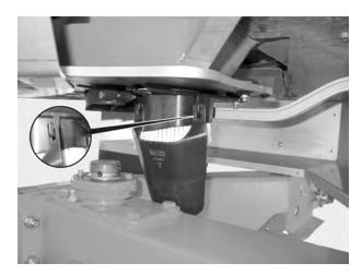
Fig. 38: Attaching the calibration test chute
