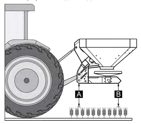
Fig. 16: Mounting position and height during normal fertilizing
