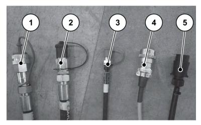
Fig. 12: Connection cables for the mineral fertilizer spreader
