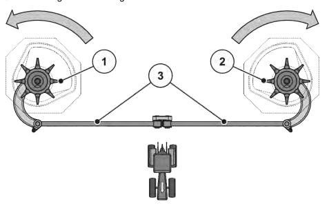
Fig. 54: Checking the agitator drive
