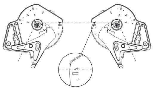
Fig. 62: Checking the drop point
