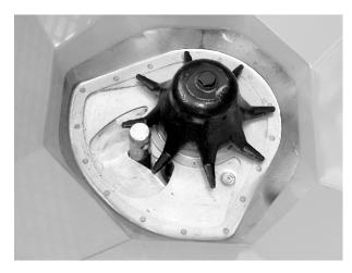
Fig. 59: Lower link pin in metering opening
