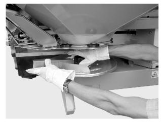
Fig. 40: Tighten the cap nut
