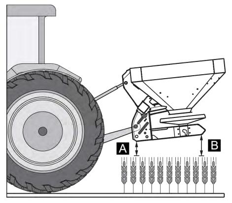
Fig. 17: Mounting position and height during late fertilizing
