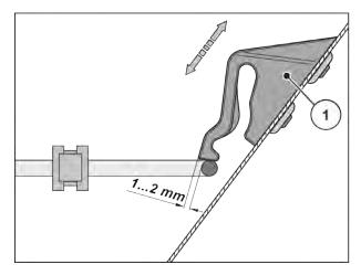
Fig. 51: Test dimensions for functional check of the protective grid interlock
