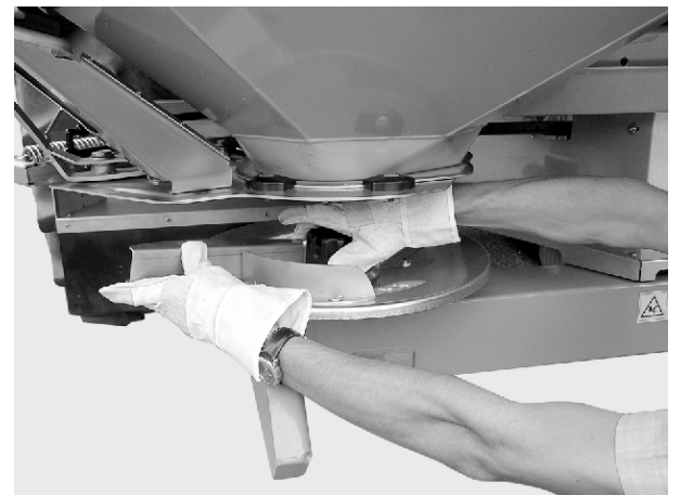
Fig. 29: Unscrew the cap nut
