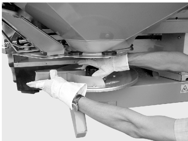
Fig. 40: Screw the cap nut on
