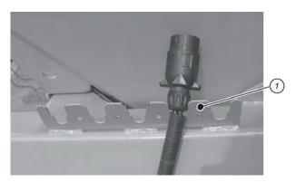
Fig. 36: Bracket for cables and hoses
