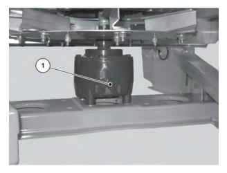
Fig. 49: Checking screw for transmission oil level
