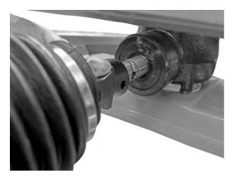
Fig. 16: Pushing the universal drive shaft onto the transmission spigot
