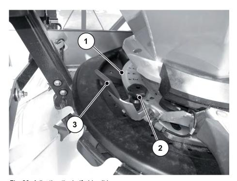
Fig. 30: Adjusting the half-side slide
