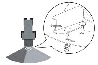
Fig. 33: Spreading density on the right in direction of travel
