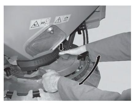
Fig. 28: Drop point adjustment center
