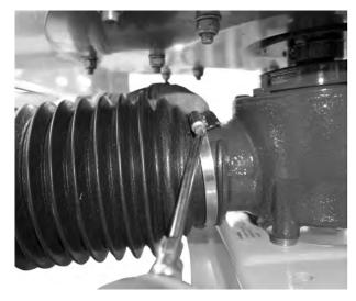
Fig. 18: Mounting the universal drive shaft guard
