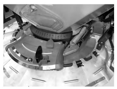
Fig. 35: Metering slider open, hydraulic cylinder on end stop
