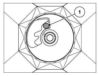
Fig. 38: Pin in the metering slide opening
