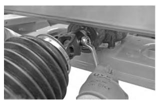
Fig. 17: Connecting the universal drive shaft
