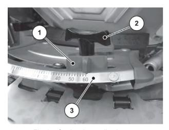
Fig. 25: Setting the application rate
