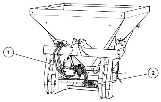
Fig. 7: Assembly overview: Hydraulic drive
