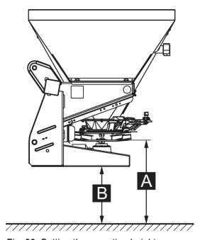
Fig. 20: Setting the mounting height
