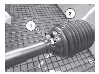
Fig. 15: Opening the universal drive shaft guard
