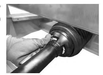
Fig. 19: Securing the universal drive shaft cover
