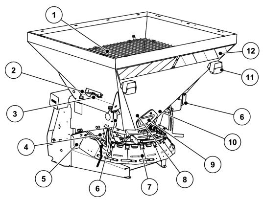
Fig. 3: Position of safety equipment, warning and instruction notices and reflector - rear
