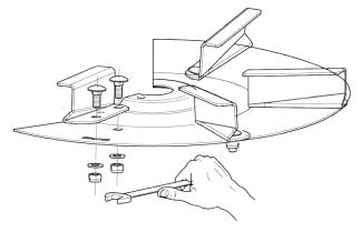
Fig. 47: Loosening the screws of the spreading vane
