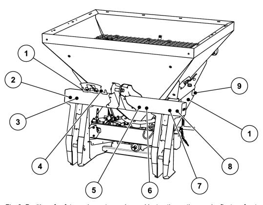
Fig. 2: Position of safety equipment, warning and instruction notices and reflector - front
