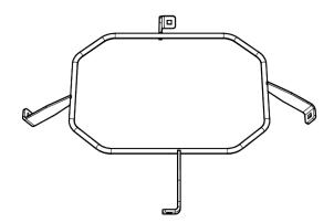
Fig. 46: Stop ring in the hopper
