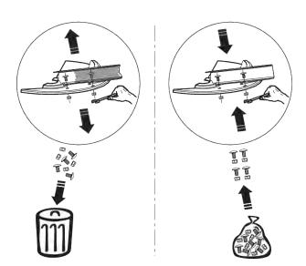
Fig. 48: Using new self-locking nuts
