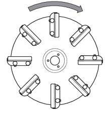
Fig. 31: Rotational direction of spreading disc
