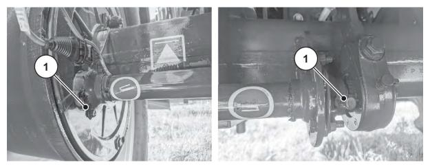
Fig. 61: Rigid axle brake camshaft bearing
