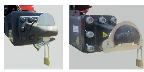
Fig. 14: Securing to prevent unauthorized use on trailer units
