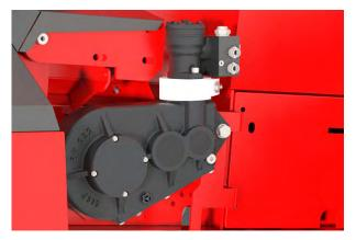
*Fig. 66: Checking the motor and the hydraulic block of the conveyor belt drive*
