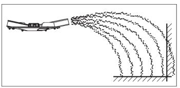
Example of full border spreading during normal fertilizing
