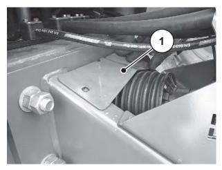
Fig. 21: Assemble the protective sheet
