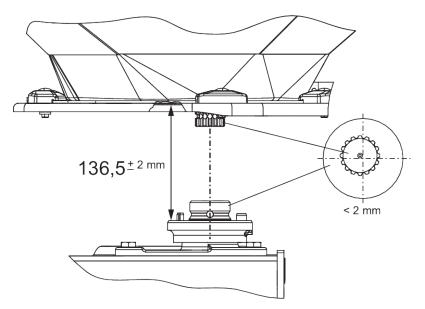
Fig. 84: Checking the position of the spreading disc hub
