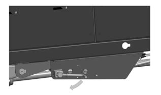
Fig. 29: Manual parking brake is closed
