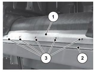
Fig. 74: Disassembling the clamping plate
