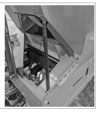
Put the adjustment lever back into the designated bracket.
