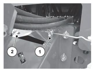
Fig. 18: Removing the protective sheet
