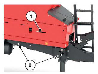
Fig. 58: Lubrication point of belt drive and towing bar
