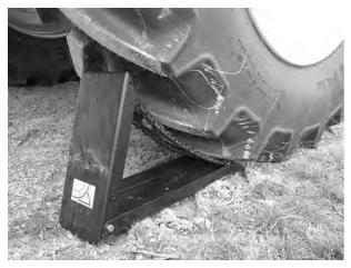
Fig. 48: Positioning the wheel chock
