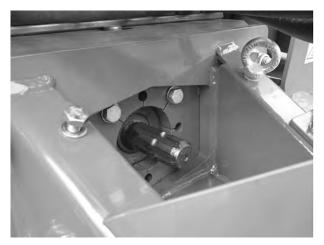
Fig. 19: Greasing the transmission spigot
