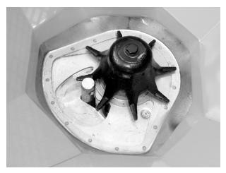
Fig. 87: Lower link pin in metering opening
