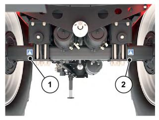
Fig. 81: Lifting jack application points
