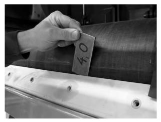
Fig. 75: Checking the clearance
