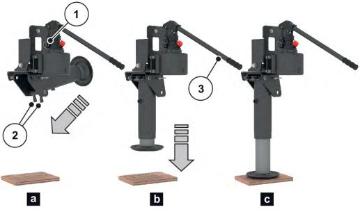
Fig. 49: Folding out the support stand
