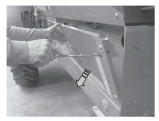
Fig. 53: Folding open the side cover
