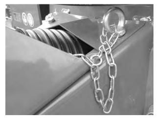
Fig. 22: Securing the safety chain
