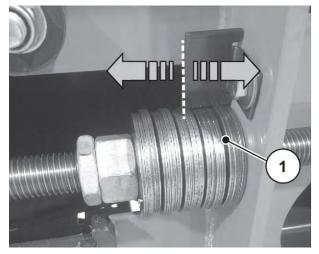
Fig. 73: Adjusting the disc spring assemblies
