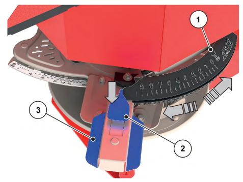
Fig. 42: Drop point adjustment center
