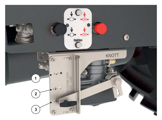
The brake force regulator is located on the frame under the manual parking brake, to the left on the side in the direction of travel.
