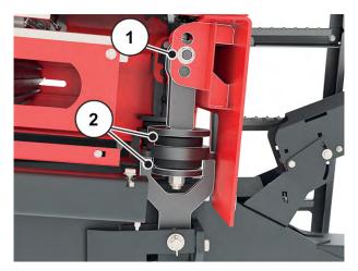
Fig. 68: Checking the towing bar suspension
