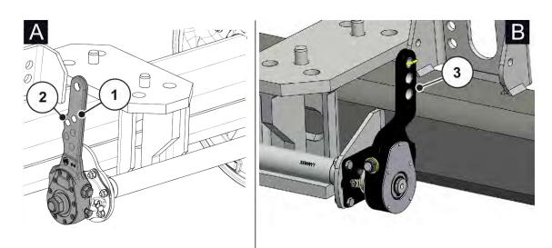
Fig. 82: Position of the brake lever/brake cylinder connection
