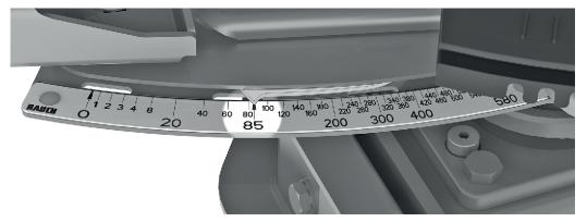
Fig. 89: Metering slide pointer on scale value 85
