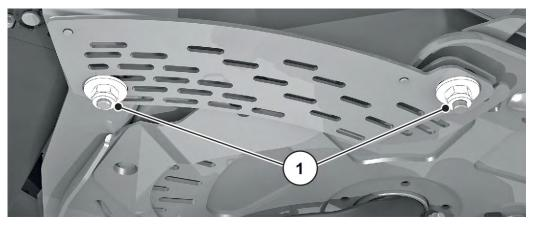
Fig. 88: Scale mounting screws
