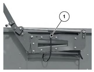
Fig. 65: Hopper cover hydraulic cylinder
