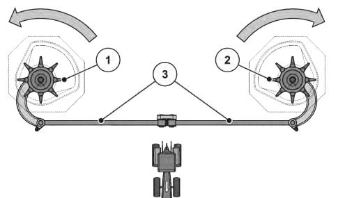
Fig. 85: Checking the agitator drive
