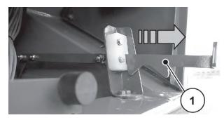
Fig. 55: Cleaning flap lever
