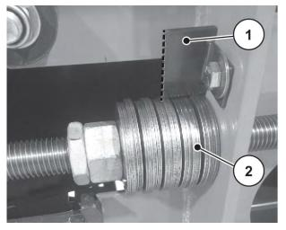
Fig. 71: Retightening the disc spring assemblies
