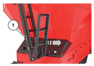
Fig. 33: Folding out the lower part of the ladder
