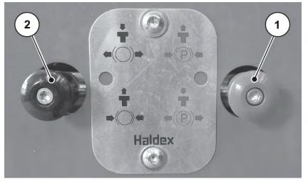
Fig. 46: Engaging the manual parking brake
