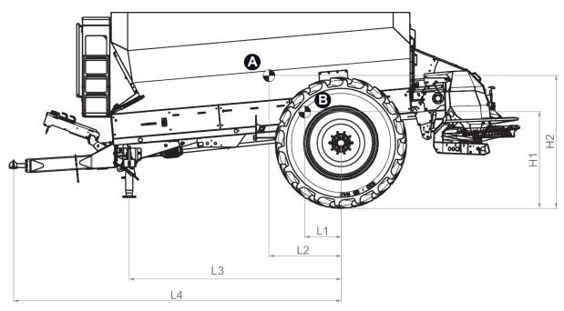
Fig. 15: Center of gravity during bottom hitching
