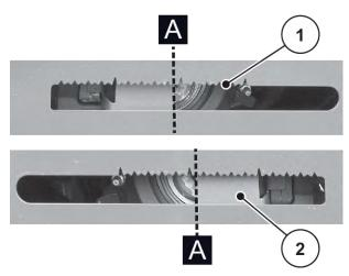
Fig. 72: Setting the disc spring assemblies
