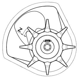
Fig. 86: Agitator head wear range
