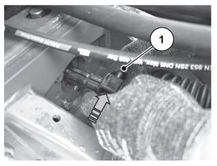
*Fig. 20: Pushing the universal drive shaft onto the transmission spigot*
