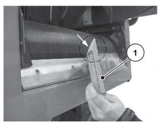
Fig. 77: Attaching the clamping plate
