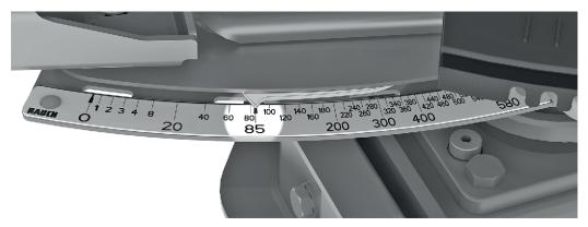
Fig. 43: Scale for displaying the application rate
