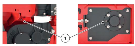
Fig. 59: Lubrication point of conveyor belt drive
