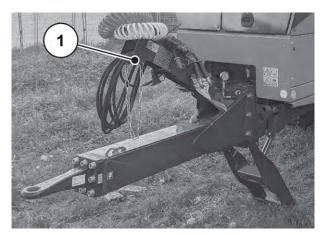
Fig. 50: PTO shaft bracket on the hose boom
