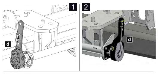
Fig. 79: Checking the free travel
