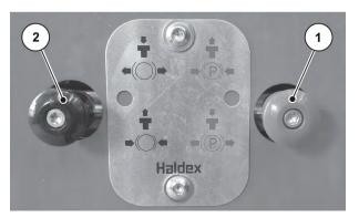
Fig. 30: Disengaging the parking brake
