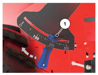
Fig. 35: Scale plate of pre-metering slide opening
