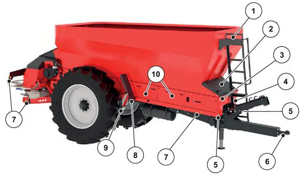
Fig. 2: Safety equipment, warning and instruction stickers, front
