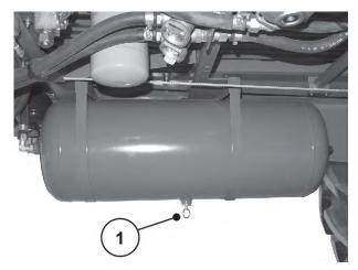
Fig. 80: Draining the air tank
