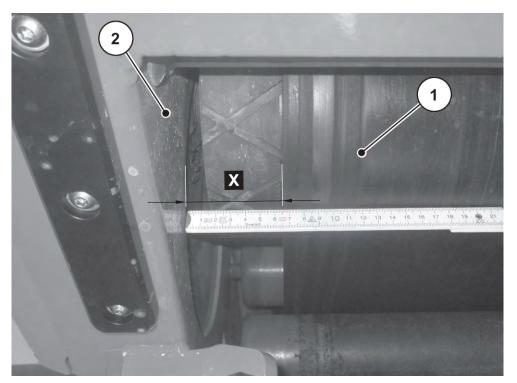
Fig. 69: Checking the position of the conveyor belt
