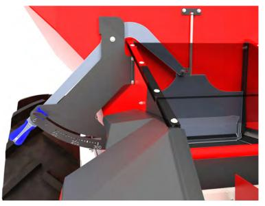
Fig. 31: Pre-metering slide in closed position
