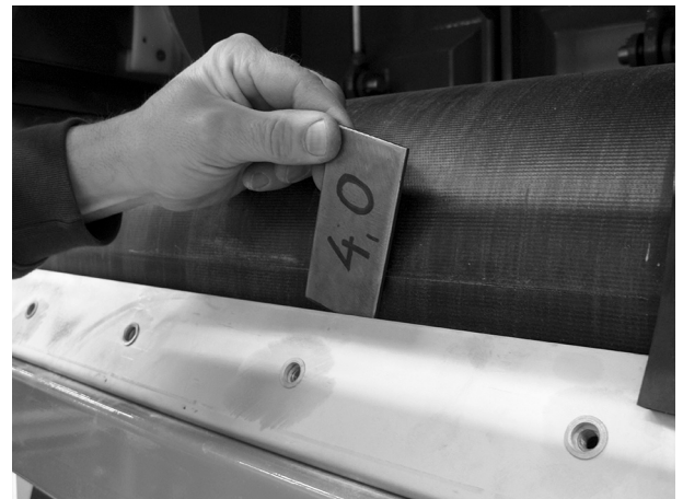
Fig. 65: Checking the clearance
