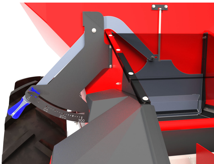
Fig. 29: Pre-metering slide in closed position
