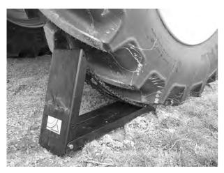
Fig. 82: Positioning the wheel chock
