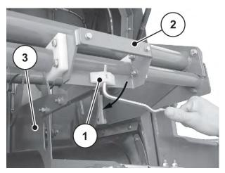
Fig. 37: Disassembling the partition plate
