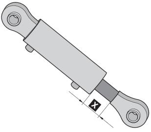
Fig. 121: Extending the piston rod
