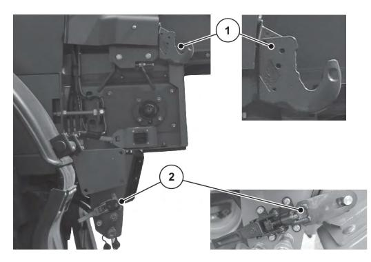
Fig. 45: AXENT 100.1 coupling points
