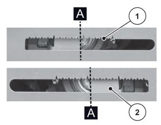
Fig. 126: Setting the disc spring assemblies
