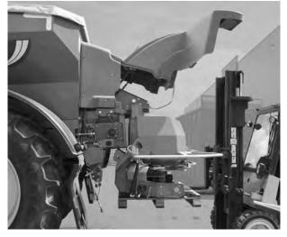
Fig. 46: Positioning the forklift truck
