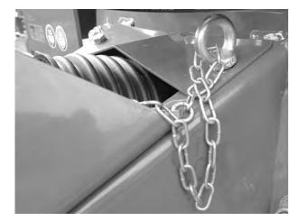
Fig. 25: Securing the safety chain
