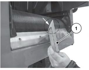
Fig. 131: Attaching the clamping plate
