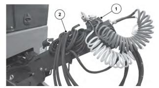
Fig. 87: Transport bracket for cables, hydraulic hoses and pneumatic lines
