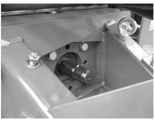
Fig. 22: Greasing the transmission spigot
