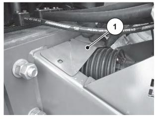
Fig. 24: Assemble the protective sheet
