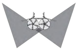
Fig. 78: Not enough fertilizer or lime in the center
