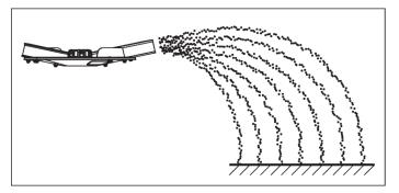
Fig. 64: Field spreading during normal fertilizing
