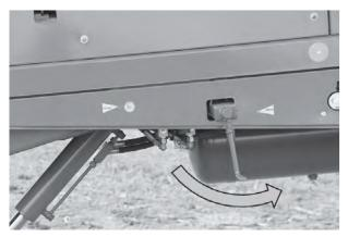
Fig. 34: Releasing the manual parking brake
