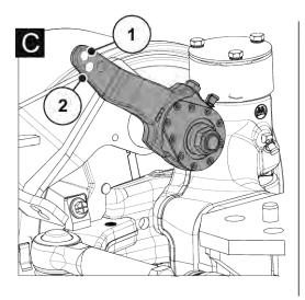
Fig. 137: Position of the brake lever/brake cylinder connection - steering axle
