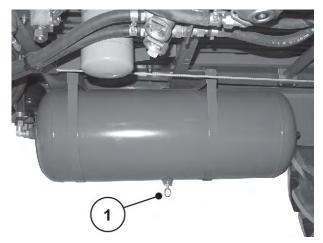
Fig. 134: Draining the air tank
