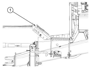
Fig. 116: Adjustment lever
