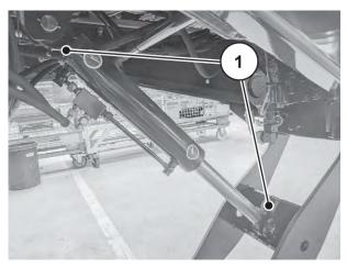
Fig. 95: Support stand hydraulic cylinder
