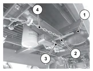
*Fig. 32: Breakaway protection of the hydraulic brake system*
