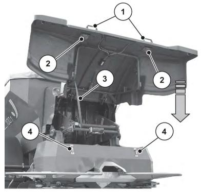
Fig. 61: Safety hood components
