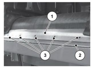
Fig. 128: Disassembling the clamping plate
