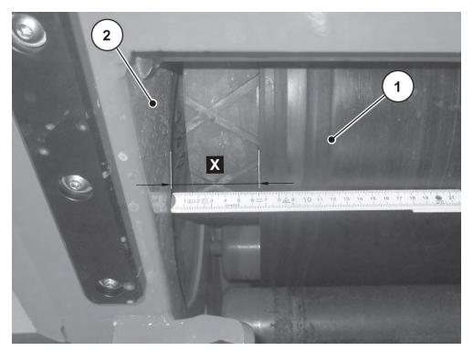
Fig. 123: Checking the position of the conveyor belt
