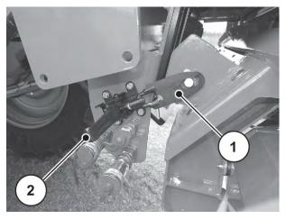
Fig. 47: Securing the spreading unit at the base
