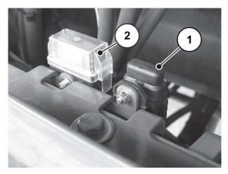
Fig. 106: Fuses at the ISOBUS cable
