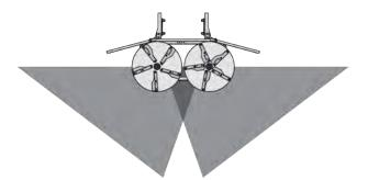
Fig. 75: Normal spreading pattern, drop point in the neutral position
