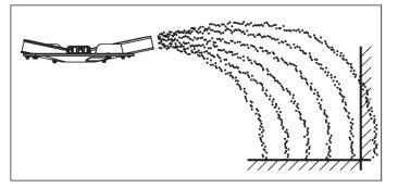
Fig. 66: Full border spreading during normal fertilizing
