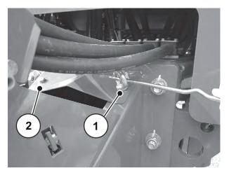
Fig. 21: Removing the protective sheet
