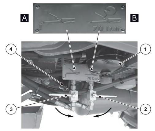
Fig. 118: Setting the towing bar suspension
