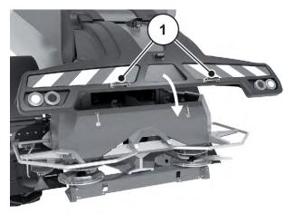
Fig. 63: Closing the safety hood
