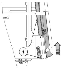
Fig. 58: Securing the sliding element
