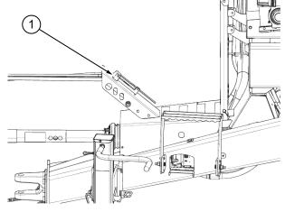
Fig. 35: Adjustment lever
