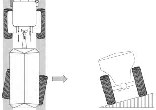
Fig. 74: Kingpin steering (optional equipment)
