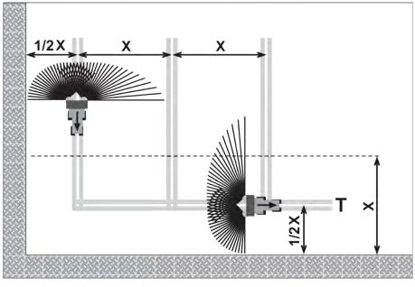
*Fig. 72: Limited border spreading* [[T]] Headland track
