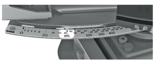
Fig. 71: Scale for displaying the application rate
