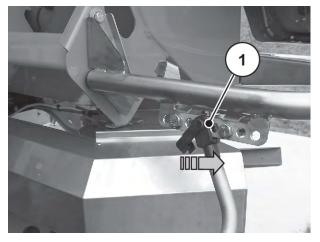
Fig. 49: Mount the mud guard extension
