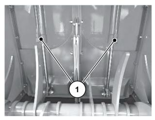
Fig. 108: Pre-metering slide hydraulic cylinder
