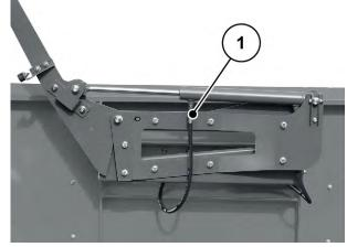
Fig. 109: Hopper cover hydraulic cylinder
