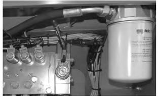
Fig. 112: Control block oil filter
