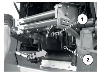
Fig. 38: Assembling the partition plate
