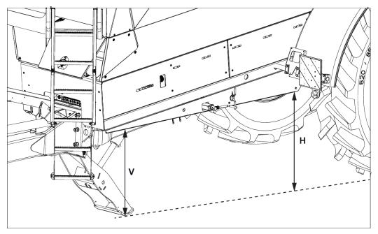
Fig. 119: Checking the machine inclination
