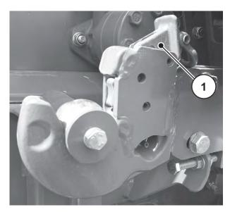
Fig. 51: Releasing the coupling points
