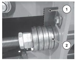
Fig. 125: Retightening the disc spring assemblies
