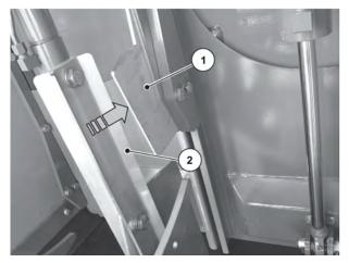
*Fig. 39: Inserting the partition plate into the guide*[1] Metal sheet guide [2] Guide holder
