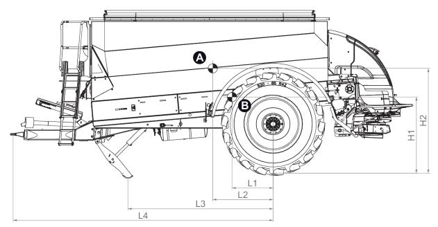
Fig. 17: Centre of gravity position for bottom hitching, rear axle position
