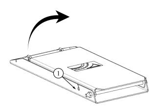
Fig. 81: Fold out the wheel chock
