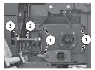
Fig. 124: Drive roller position
