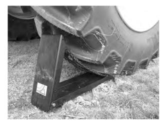
Fig. 86: Positioning the wheel chock
