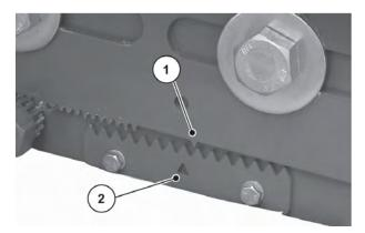
Fig. 76: Drop point in the neutral position
