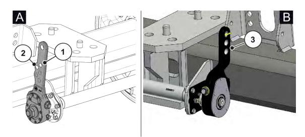
Fig. 136: Position of the brake lever/brake cylinder connection - rigid axle
