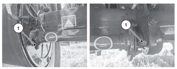
Fig. 99: Rigid axle brake camshaft bearing
