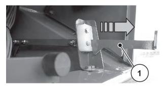
Fig. 91: Cleaning flap lever
