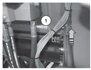
Fig. 53: Cleaning flap in closed position, front in direction of travel
