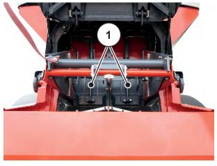
Fig. 52: Pre-metering slide in closed position
