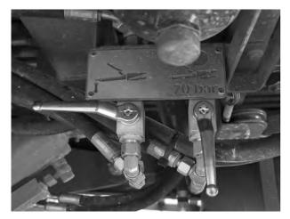
Fig. 120: Close the left shut-off valve.
