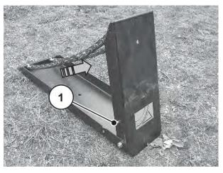
Fig. 85: Fold out the wheel chock
