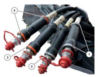
Fig. 27: Marking of the hydraulic hoses
