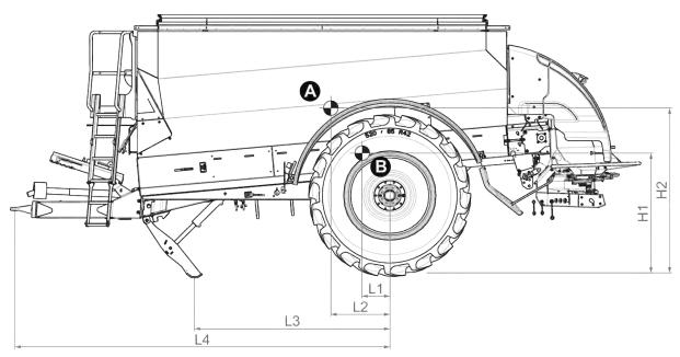
Fig. 16: Centre of gravity position for bottom hitching, front axle position
