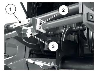
Fig. 40: Securing the partition plate
