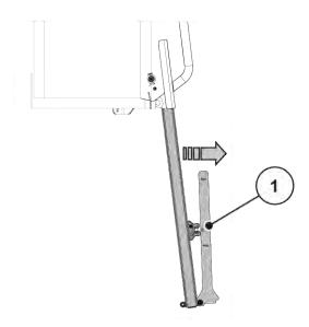
Fig. 56: Folding out the bottom part of the steps
