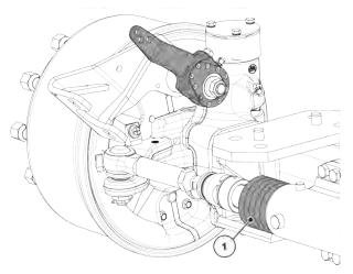
Fig. 114: Distance washers of the steering axle
