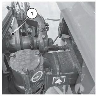
Fig. 100: Steering axle brake camshaft bearing
