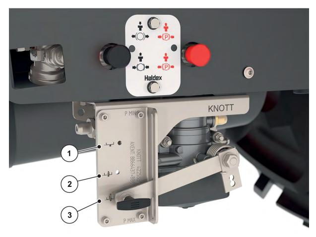
Fig. 31: Brake force regulator setting
