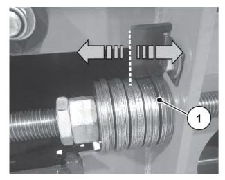
Fig. 127: Adjusting the disc spring assemblies
