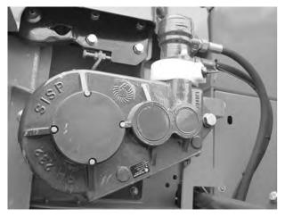
Fig. 110: Checking the conveyor belt motor
