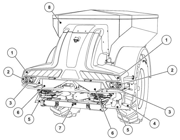
Fig. 3: Safety equipment, warning and instruction stickers, rear
