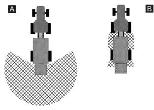
Fig. 1: Hazard zone when devices are pulled
