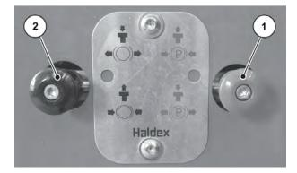
Fig. 33: Disengaging the parking brake
