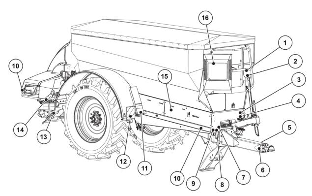
Fig. 2: Safety equipment, warning and instruction stickers, front
