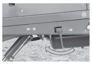
Fig. 84: Engaging the manual parking brake
