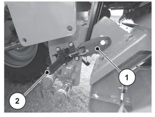
Fig. 50: Releasing the spreading unit at the bottom
