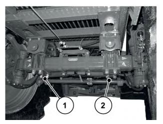
Fig. 135: Lifting jack application points
