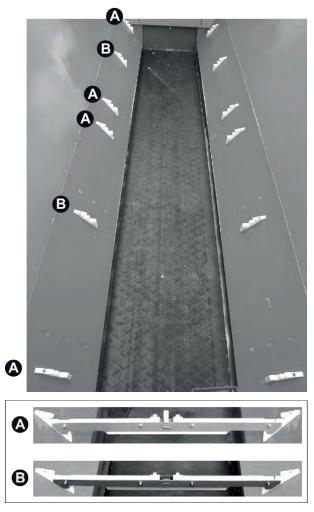
Fig. 41: Installing the bracket of the feeder mesh
