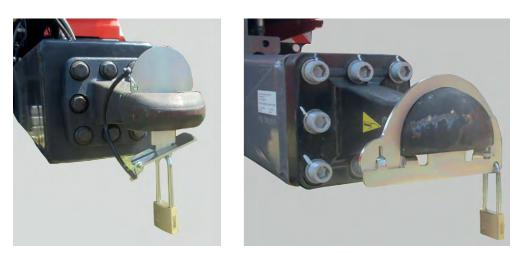
Fig. 12: Securing to prevent unauthorized use on trailer units
