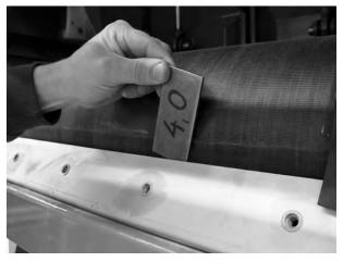
Fig. 129: Checking the clearance
