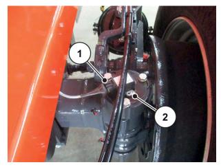
Fig. 115: Axle angle sensor
