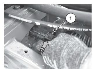
*Fig. 23: Pushing the universal drive shaft onto the transmission spigot*
