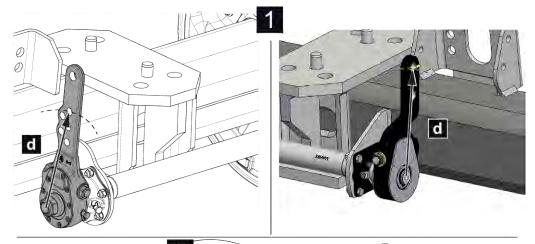
If the braking effect is reduced and the free travel exceeds 10 - 15% of the brake lever length [d], the slack adjuster must be adjusted by your specialist workshop.
