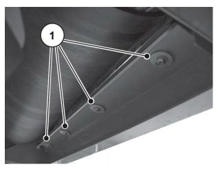
Fig. 130: Adjusting the position of the bracket
